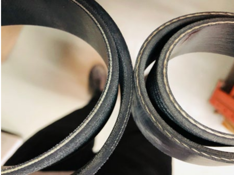
Defective Aramid cord reinforced belt (left) vs New polyester cord belt (right) – Note the different cord arrangement between the two belt types.
