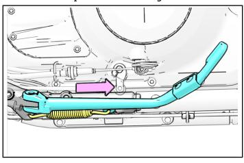
6. Swing sidestand to the extended position to align bolt hole and install bolt and nut.
