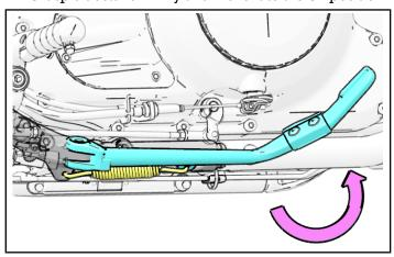
5. Grasp sidestand firmly. Pull sidestand rearward against spring tension until mounting flange on sidestand is clear of the mounting boss on the frame.
