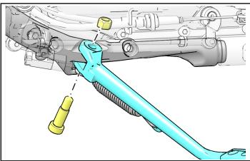
7. Torque to specification and wipe off any excess grease.
