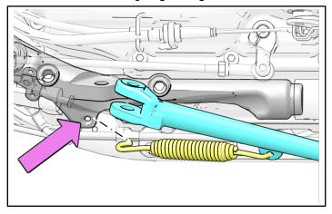
With sidestand in the retracted position (up) grasp sidestand firmly and, pull stand rearward against spring tension until the mounting flange on the sidestand drops onto the mounting boss on the frame.
