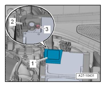
Disconnect the 12V battery with the ignition switched ON:
