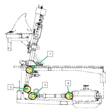
Figure 1: Locations to Torque on Steering System
