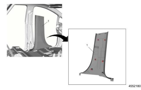
28. Install the Center Pillar Lower Trim Panel (1) on both sides of the vehicle.
