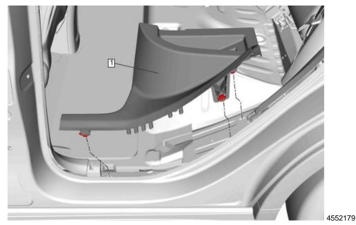
34. Install the Rear Side Door Sill Garnish Molding on both sides of the vehicle.
