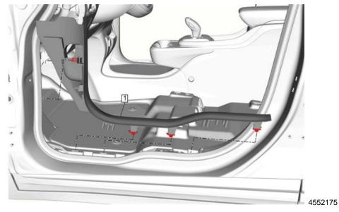
29. Install the Front Side Door Sill Garnish Molding (1) on both sides of the vehicle.
