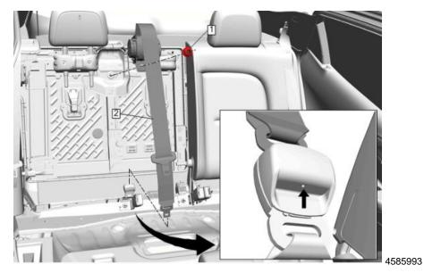
1. Push pin in the slot on mini-buckle to disengage the rear center seat belt retractor from the rear center seat belt buckle.
