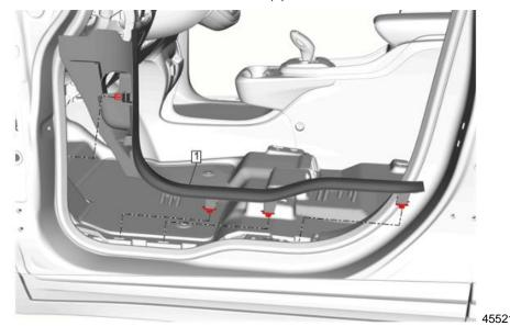
35. Install the Front Side Door Sill Garnish Molding (1) on both sides of the vehicle.
