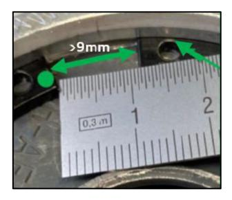
• Check circlip on left (driver) front air spring strut and replace strut, if necessary.
