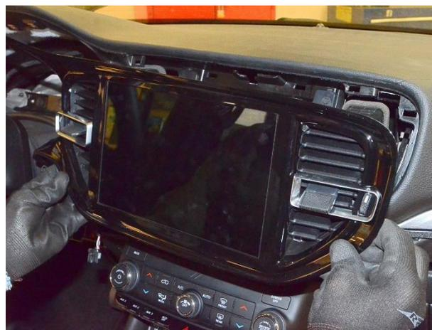
**Figure 28 – Radio Display and Bezel**
