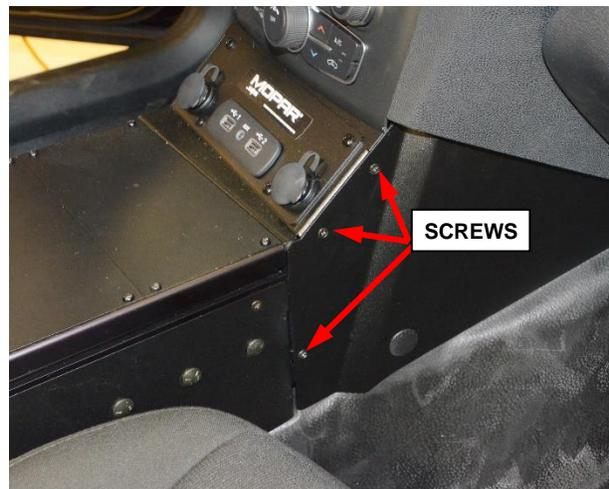
Figure 1 – Console Side Cover Screws
