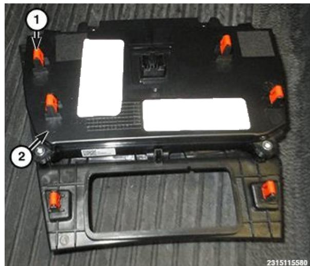
**Figure 4 – HVAC Control Retainers**
