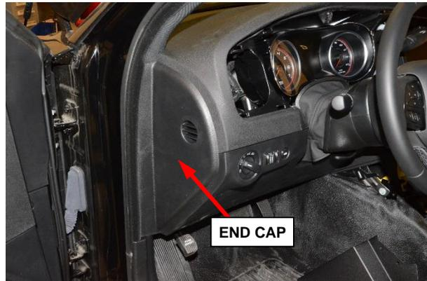
**Figure 5 – Instrument Panel End Cap**
