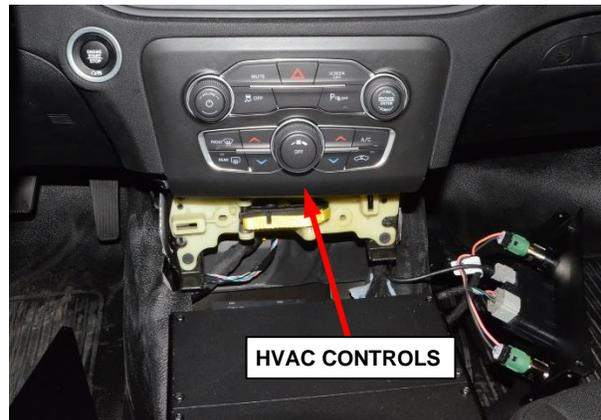
**Figure 3 – HVAC Controls**
