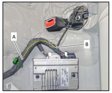
Open and unwrap the wiring harness starting at the branch <A> and continue to branch <B>.
