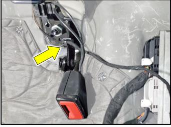
Clip the seat belt wiring harness to bracket at <arrow>.
