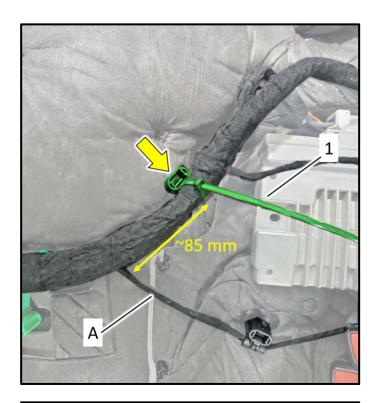
Install new tie wrap <1> around wiring harness and through stud clip <arrow>.
