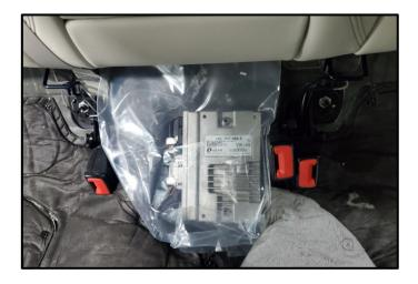
Install protective cover over Gateway Control Module.
