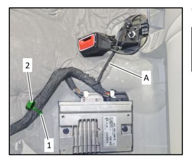
Vehicles with additional wiring to right rear seat belt buckle from the gateway:
