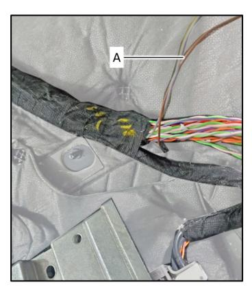
Separate the two wires <A> for the right rear seat belt buckle.
