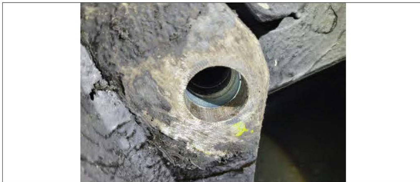
Figure 4 - Clean the Surface for the Nord-Lock Washer
