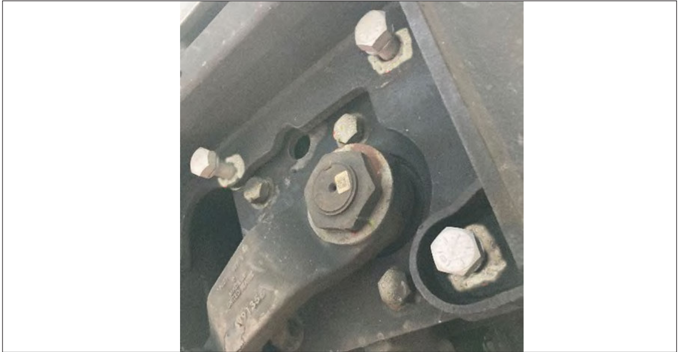
Figure 7 - Install Bolts (Do Not Torque)
