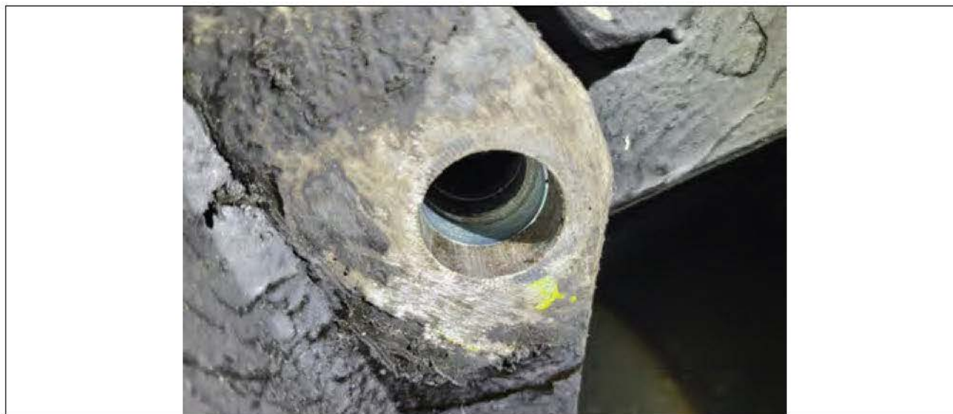
Figure 4 - Clean the Surface for the Nord-Lock Washer
