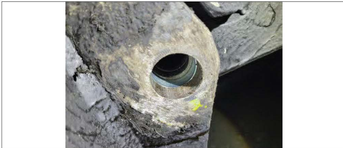
Figure 4 - Clean the Surface for the Nord-Lock Washer
