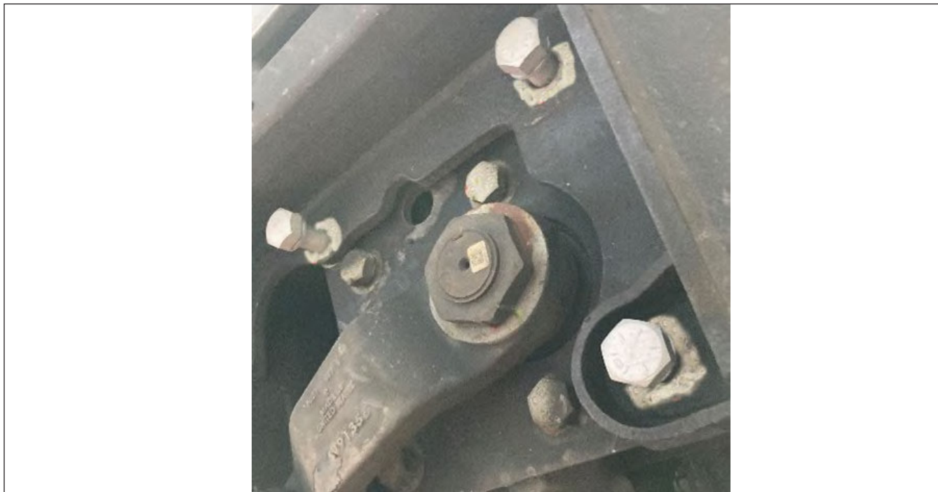
Figure 7 - Install Bolts (Do Not Torque)
