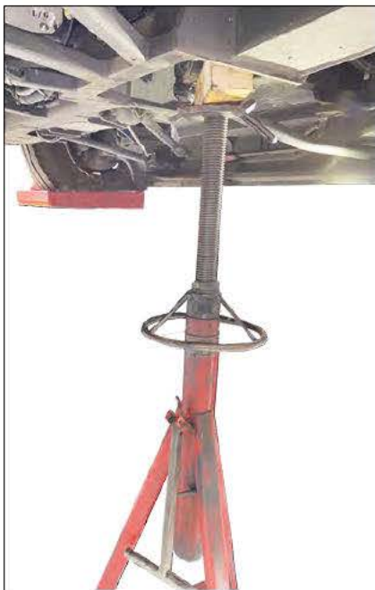
Figure 5 - Use a Jack Stand to Lift Slightly the Gear Box Mounting Plate
