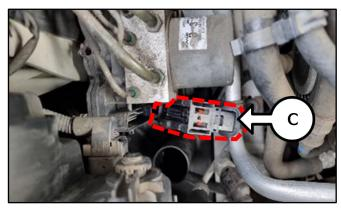
3. Inspect the HECU connector (C) and harness for signs of fluid intrusion, corrosion, and melting.
