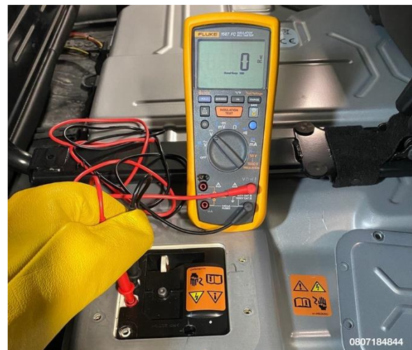
Figure 6 – Measuring at High Voltage Test Points
