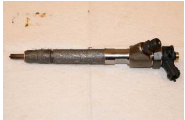
Figure 147 – Lubricate the Fuel Injector
