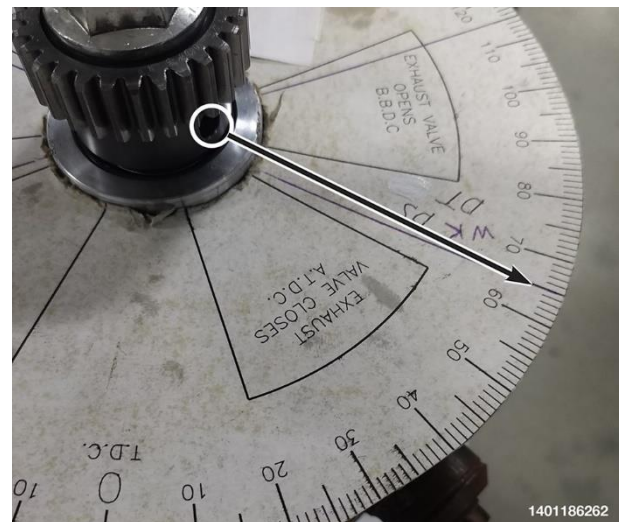
Figure 199 – Installing a Printed Paper Degree Wheel from the Internet
