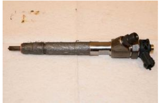
Figure 52 – Lubricate the Fuel Injector
