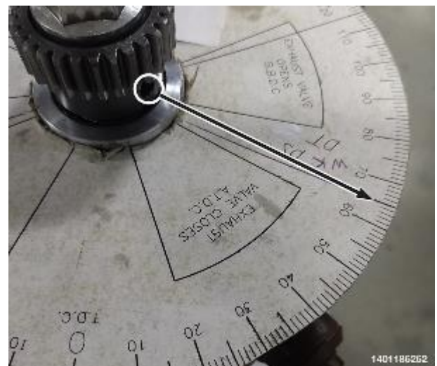
Figure 169 – Installing a Printed Paper Degree Wheel from the Internet
