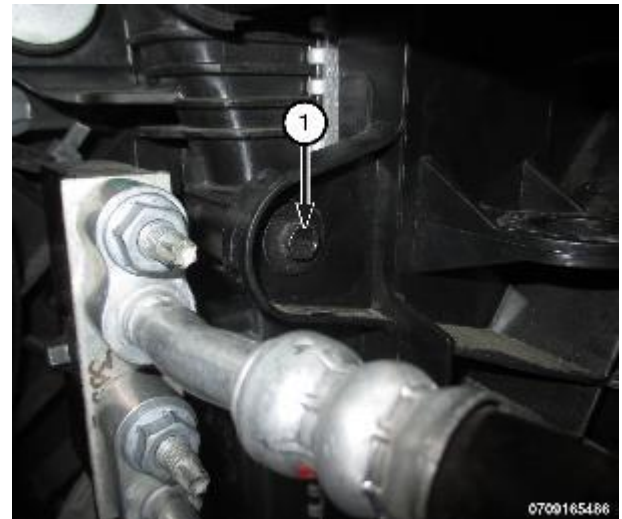
Figure 95 – Left Cooling Fan Bolt
