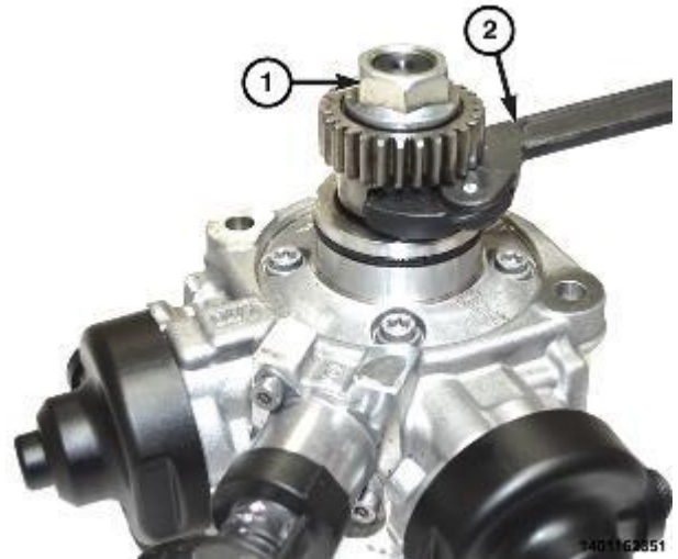
Figure 170 – Installing the Drive Gear on the HPFP
