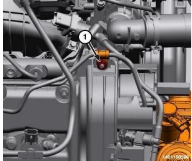
Figure 56 – High Pressure Fuel Tube Bolt
