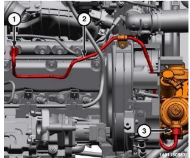
Figure 20 – Right Bank Fuel Supply
