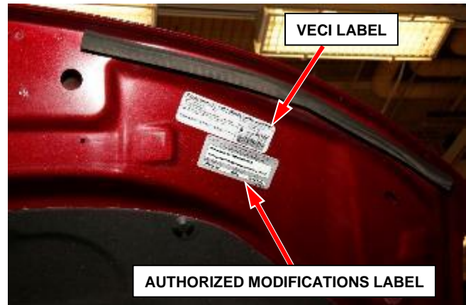
Figure 199 – Apply Authorized Modifications Label Near VECI Label (Specific Vehicle May Look Different)
