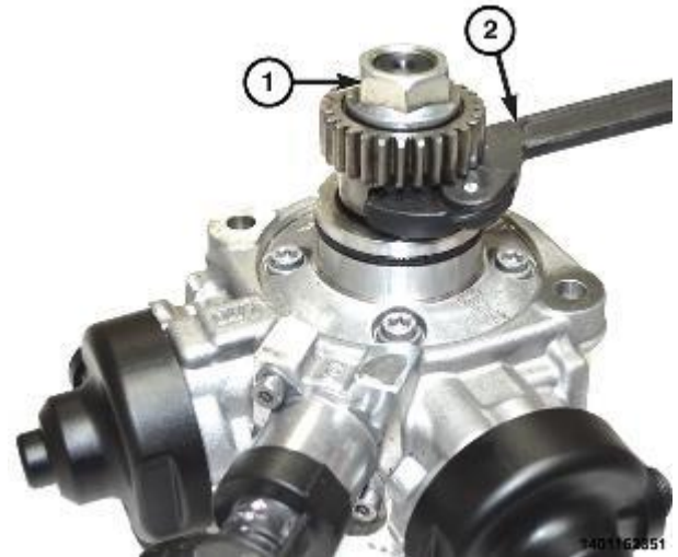
Figure 170 – Installing the Drive Gear on the HPFP
