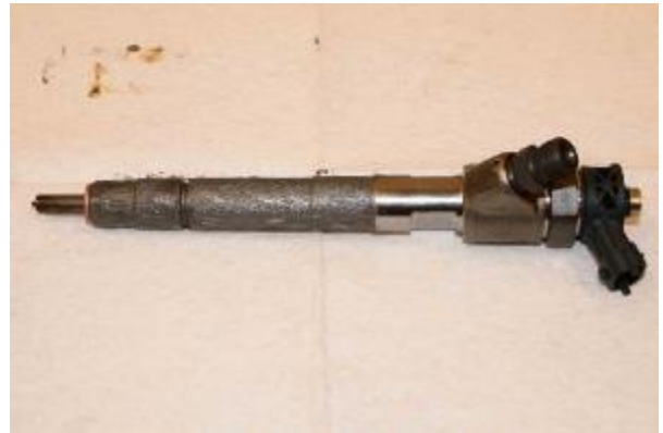
Figure 142 – Lubricate the Fuel Injector
