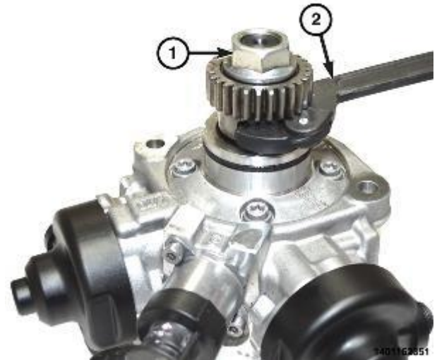
Figure 193 – Gear Nut Removal
