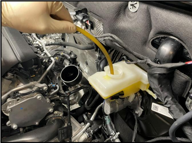
**Remove brake fluid from reservoir:**
