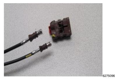
• Remove the two coax cables from the connector.
