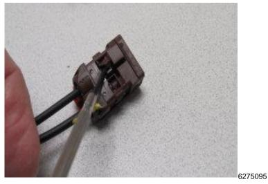
Slightly lift the retention tabs, releasing the coax cables from the connector.
