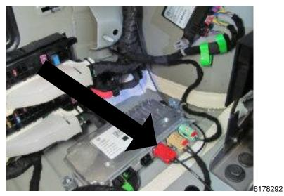
18. Starting with the red connector at the VPM, route the new coax cable.
