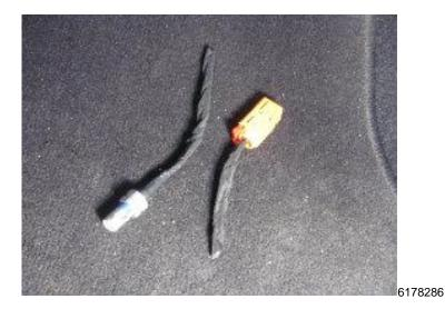
Note: Ensure that you service the orange VPM connector, not the radio coax.
