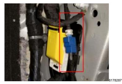
15. Locate the coax cable that goes from the A11 radio to the X209/208 IP to Body Coax In-line Connection. Disconnect both connectors.
