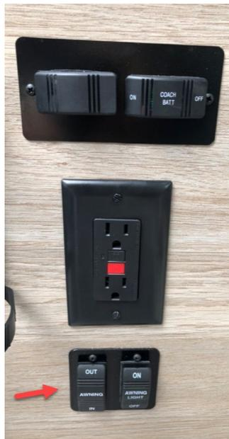
2. Remove the 2 switches from panel and label awning light switch connector for reinstallation. **NOTE: Awning in/out switch will not be used.**
