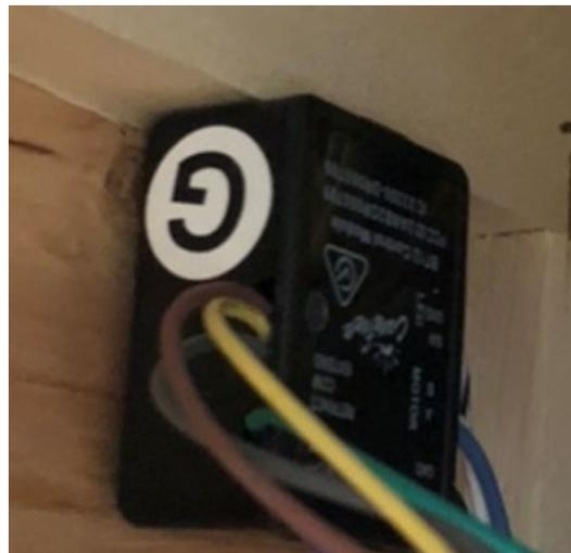
7. Remove drawer under shirt closet. Run new harness down wall and come out in bed frame behind load center. Run additional length of wiring from harness forward to the switch plate.
