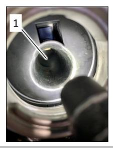
Fuel condensation formed on adapter cap <1>.
