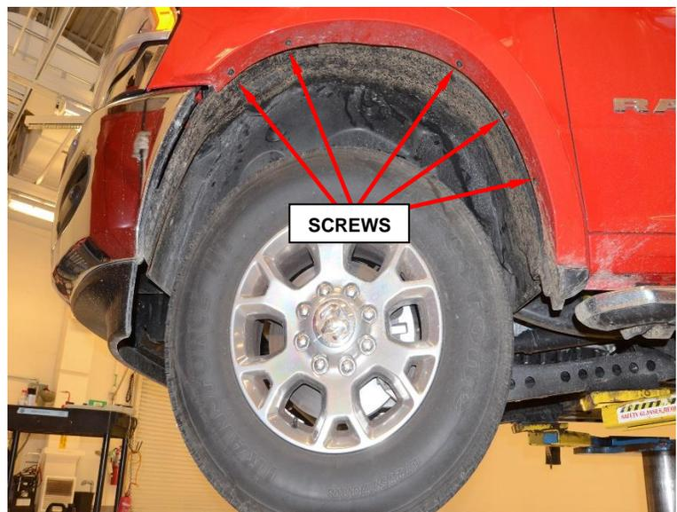
Figure 2 – Wheelhouse Splash Shield
