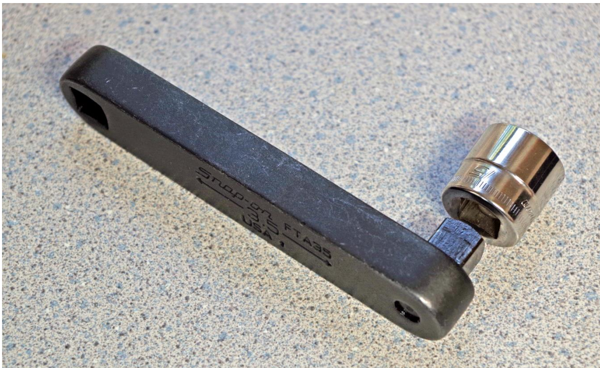
Figure 1 – 15mm Offset Wrench or Torque Adapter with Shallow Socket
