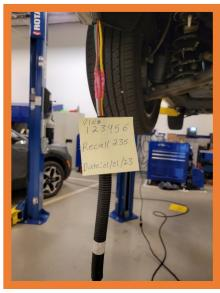
17. Raise the corrugated tube up to the mark and seal both ends with electrical tape.
