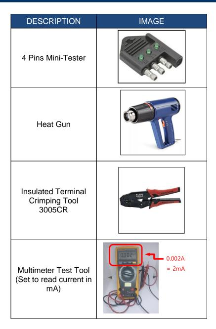
NOTE: Other crimp tools can be used (e.g. general crimping tool below), as long as it is intended for insulated wire terminals (nylon terminal).
