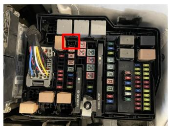
Measure both terminals where the fuse was with a 3. multimeter probe.
