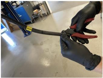
13. Strip the sheath of the wires. Expose 8-10mm of the wiring.
