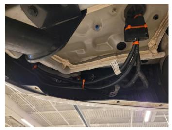
10. Route the Tow Hitch Harness over the bumper beam behind the rear bumper. Fasten and secure harness with (2) cable ties.
