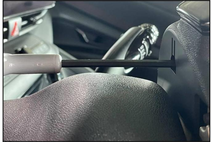
Insert the Allen wrench/screwdriver until it cannot go in any further. Gently press the end of the Allen wrench/screwdriver upward to depress the pin.
