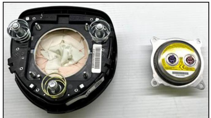
4. Deploy the airbag inflator module using the airbag deployment tool 0957A-34100A (superseded by 0957A-34100C). Refer to applicable Shop Manual for detailed instructions.
