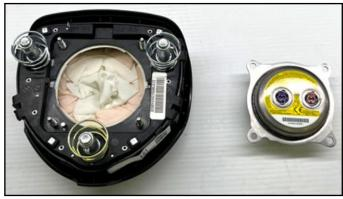
4. Deploy the airbag inflator module using the airbag deployment tool 0957A-34100A (superseded by 0957A-34100C). Refer to applicable Shop Manual for detailed instructions
