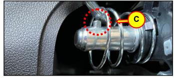
Use an H4/H5 Allen wrench/screwdriver to depress the airbag fastening pins.
