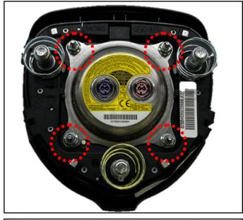
Separate the driver airbag cover from the airbag inflator module.
