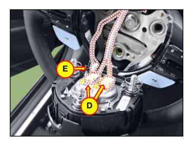
7. Remove and replace the driver airbag with a new one.
