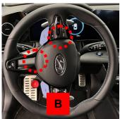
5A. To release the left and right fastening pins, insert the Allen wrench/screwdriver H4/5 in a straight parallel position as shown in the picture to the right.
