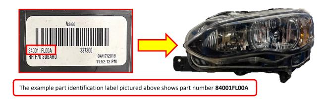
Headlamps with part number **84001FL00B** or **84001FL01B** will not require replacement and can be reinstalled and adjusted. ALL other part numbers will require replacement and adjustment.
