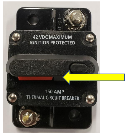
Figure 2: Bad Circuit Breaker with RED arm
