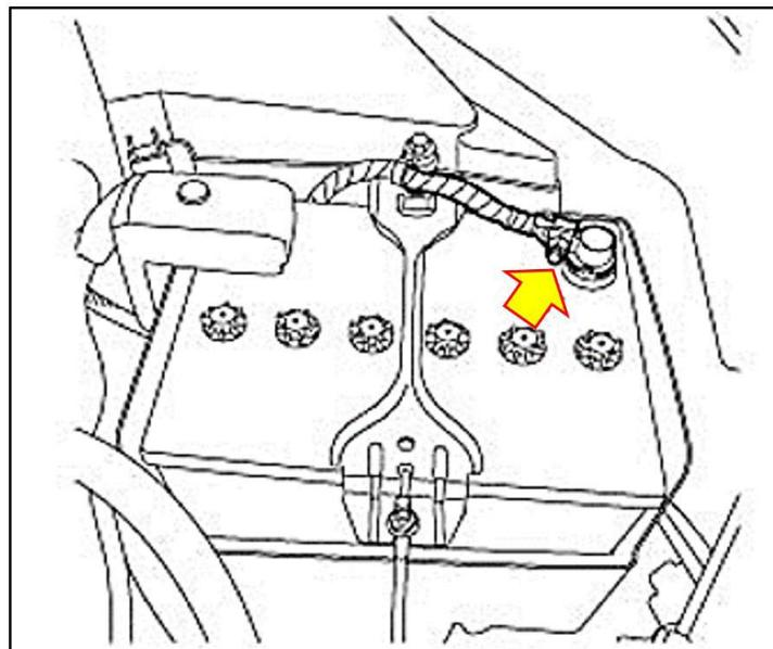
**NOTE:** If needed, clean the battery cable terminals and apply the approved protectant.
