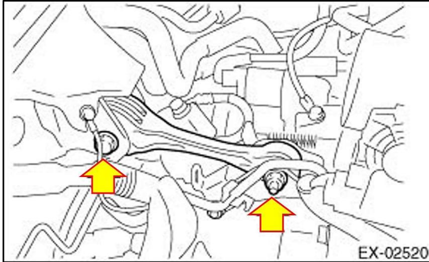
**STEP 51:** Install the nut and lock washer at the starter B connection to the starter motor and torque to **11Nm (8.1ft-lb)**.
