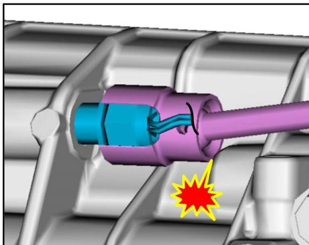
**STEP 30:** Install the new back-up switch with the new gasket. Rotate the switch by hand while turning its connector in order to avoid any twisting of the harness.
