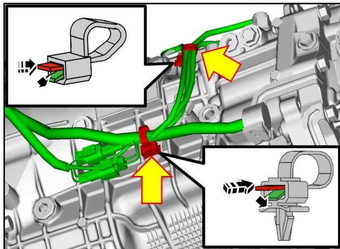
**STEP 26:** Disconnect the gray two-pin connector on the back-up switch harness.
