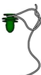
(3) Insert the clip and tie the string to the muffler bracket.
