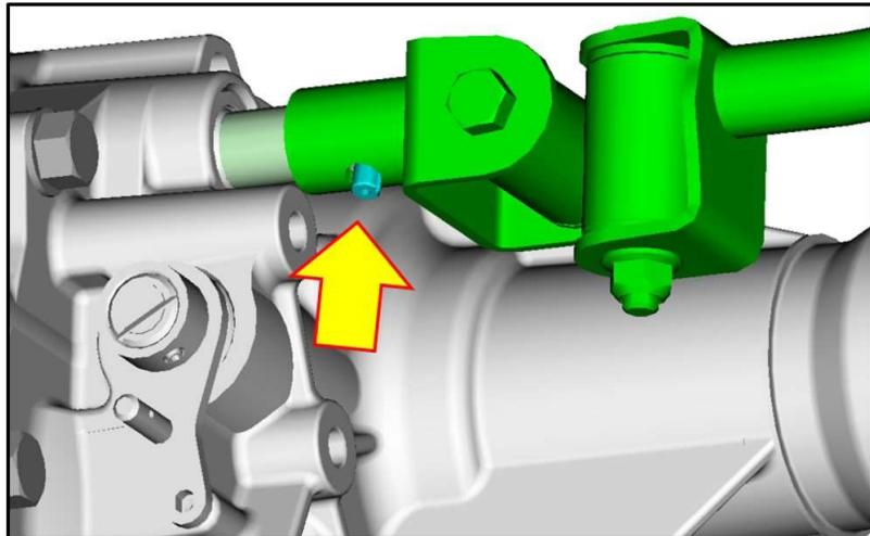
**STEP 22:** Once the spring pin is removed, the shift rod can then be positioned in the third gear (toward the front of the vehicle).
