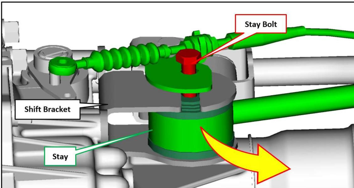
**STEP 19:** Remove the three bracket mounting bolts then remove the shift bracket.
