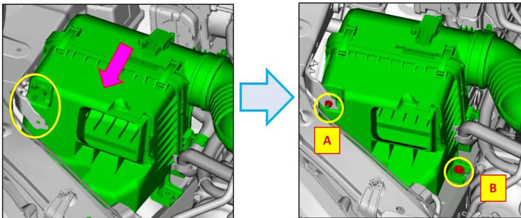
**STEP 56:** Install the air intake duct with the two mounting clips.
