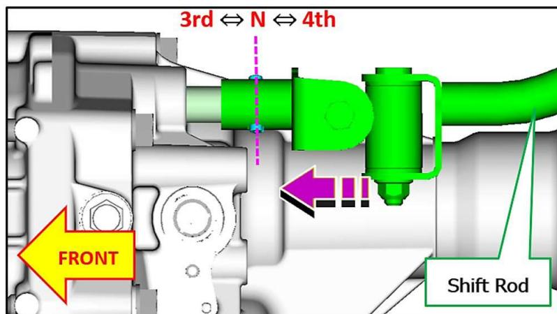
**STEP 23:** Separate the shift rod from the shifter arm shaft. Moving the shift rod in a twisting motion can make this process easier.
