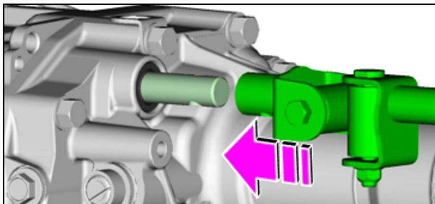
**Tip: To prevent losing the positioning clip, attach a lead using string or wire.**
