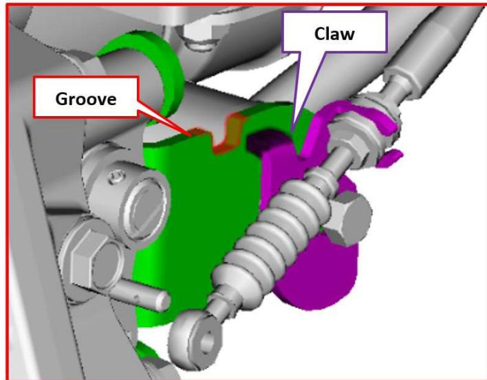
**STEP 44:** Install the reverse check cable to the reverse check lever. Secure the connection with the washer and locking snap pin.
