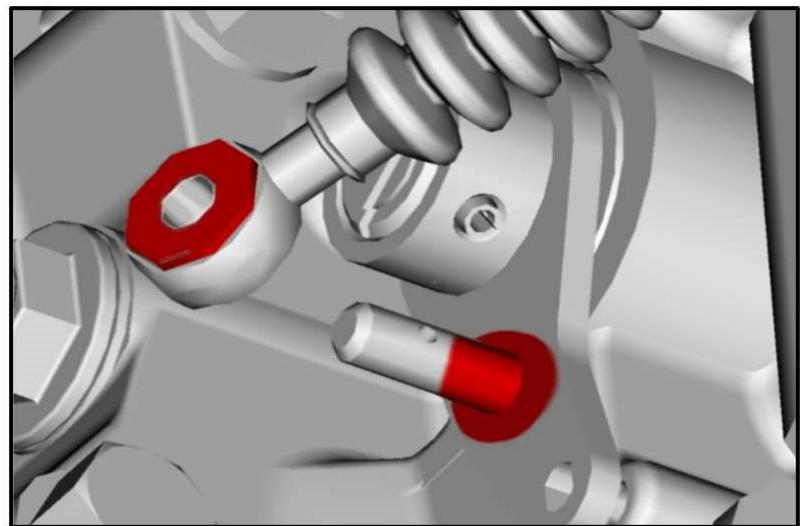
**STEP 43:** Install the stay, stay bolt, and cable plate into the shift bracket and tighten the bolt to 32Nm (23.6ft-lb).
