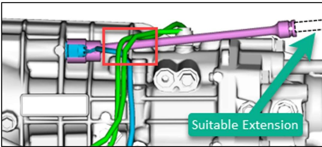
**CAUTION:** Confirm the socket is fully seated onto the back-up switch. Confirm the wires are not damaged by the socket.
