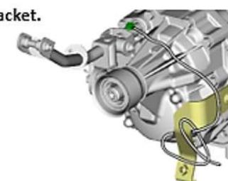
**STEP 35:** From the top side, insert the supplied positioning clip (p.n. 909130096) in the hole until the clip flange is fully seated.
