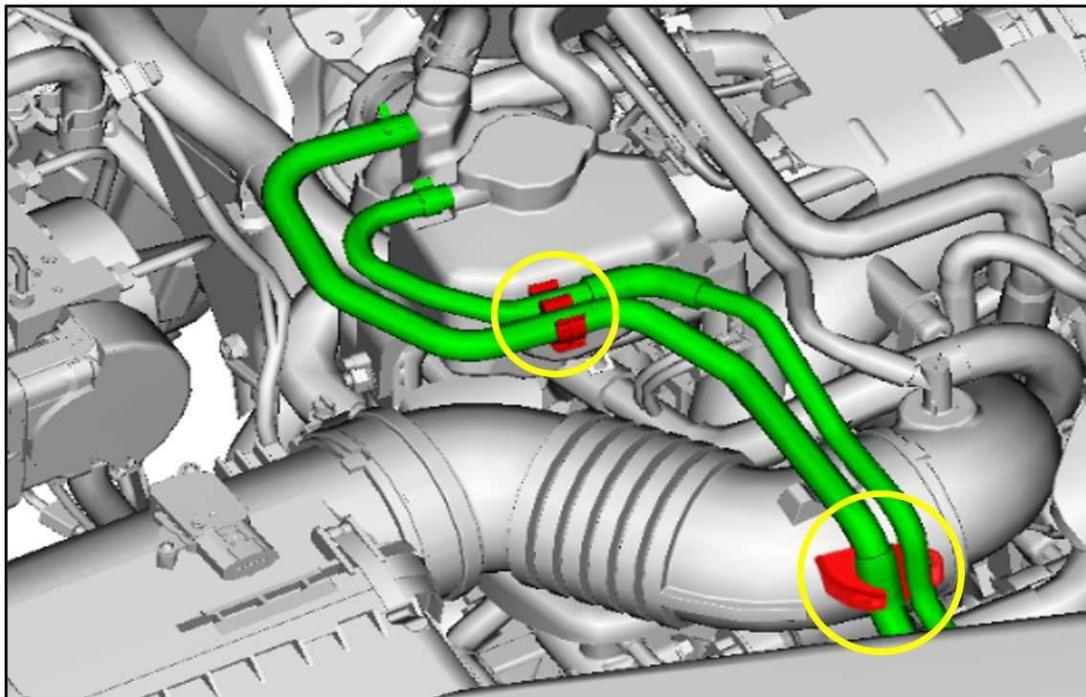
**STEP 11:** Remove the two clips retaining the air intake duct and removed the air intake duct. This will prevent the duct from interfering with the injector cover.
