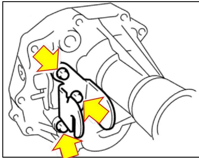
**STEP 20:** Position the shift rod in fourth gear (towards the rear of the vehicle). This will be the optimum position for removal of the spring pin.
