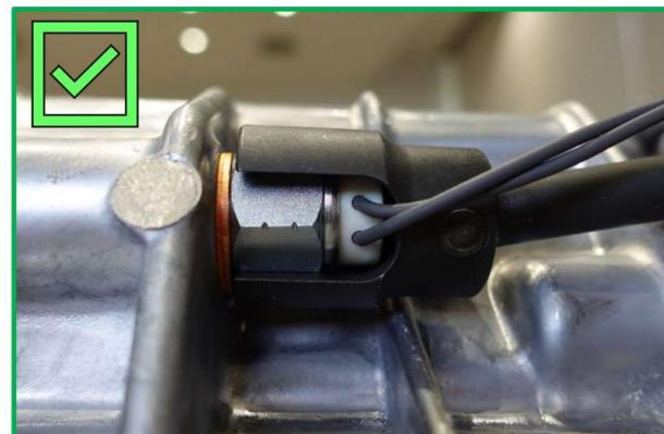
**CAUTION:** Take particular care not to damage the neutral position switch with the special tool.
