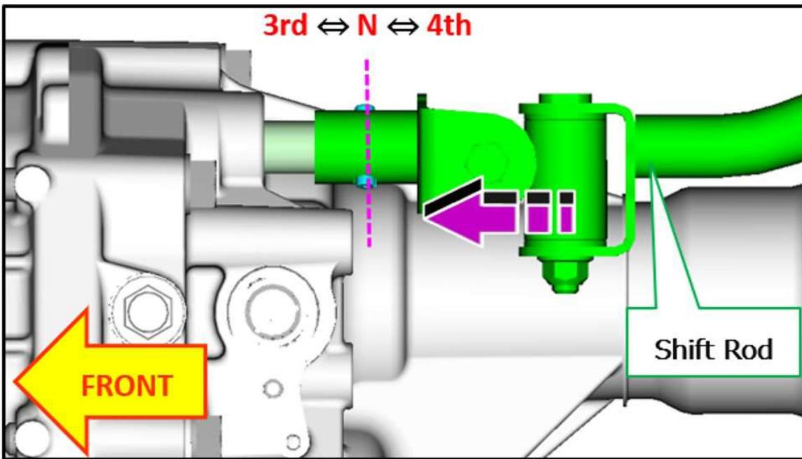
**STEP 40:** Install the shift bracket with the three mounting bolts torqued to **25Nm (18.4ft-lb)**.
