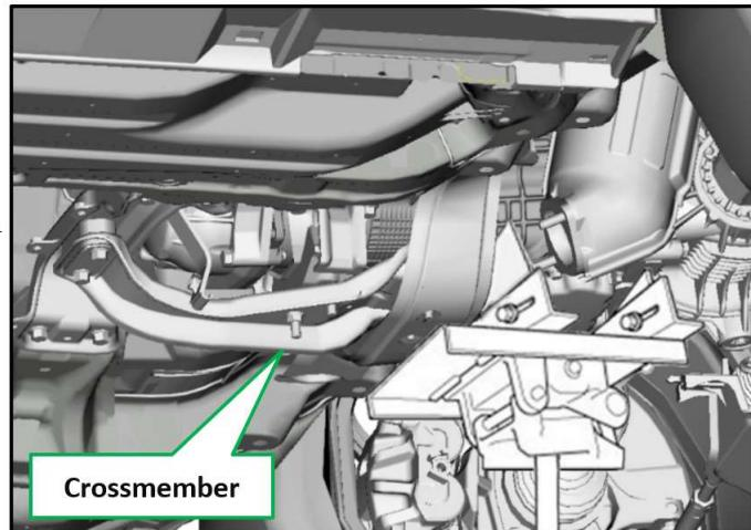
Remove the six mounting bolts and two mounting nuts. Remove the crossmember.
