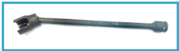
The Extension Cap (**p.n. 18678AA010**) is used to prevent any unwanted oil loss during work procedures.
