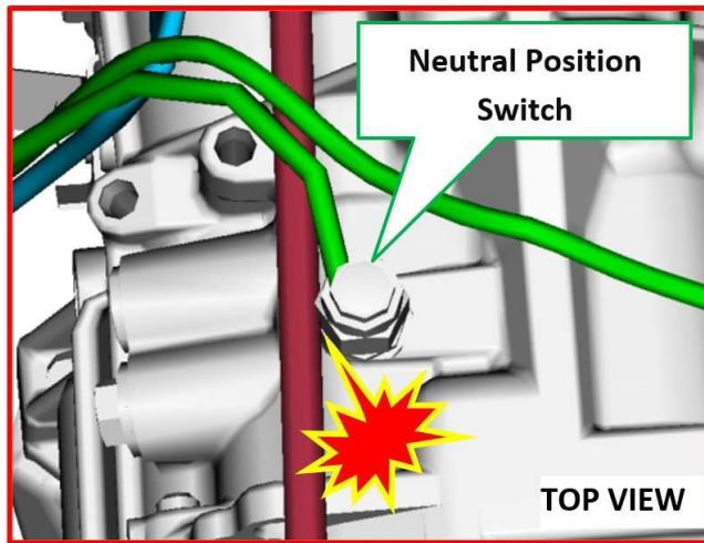
**STEP 29:** Loosen the back-up switch from the transmission case. Rotate the switch harness while turning the socket to prevent any excessive tension. The switch and the special tool cannot be removed together due to interference with the transmission case. Remove the tool before removing the switch.
