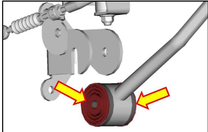
**STEP 42:** Apply a thin layer of Conoco Philips Multiplex Red #2 (**p.n. 000041000**) to the bushing of the reverse check cable its associated contact point.
