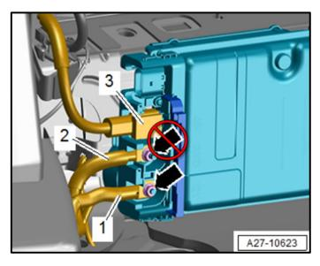
• Torque nut for cable <1> to 20 Nm.
