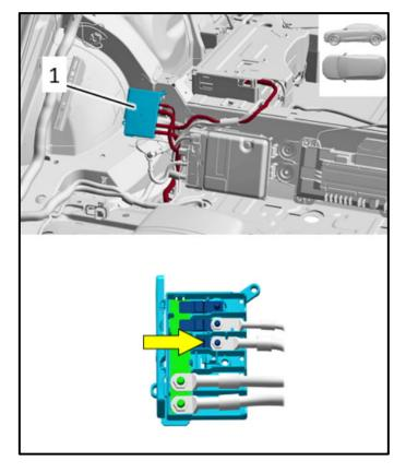
• Torque ground connection <circle> to 9 Nm.
