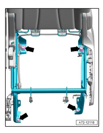
• Torque seat frame mount bolts to 50 Nm.
