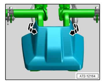
• Release the hooks <arrows> and remove the trim panel forward.
