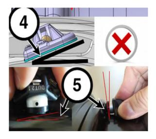
NOTE: Installation OK, flat/parallel positioning of the wheel electronics module on rim well base(6).
