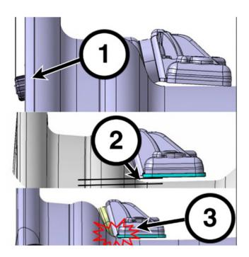
installation, a maximum protrusion of 0.098in (2.5mm) must not be exceeded (3).
