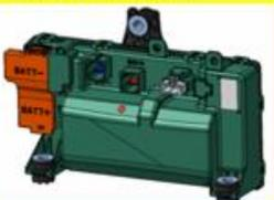
Remove each of the 2 Main Relays from the PRA as shown by these 4 steps. Pry apart each tab and hold both apart with wire ties inserted, then pull up the relay. **Please retain the main relays. They are subject to WTC callback.**
