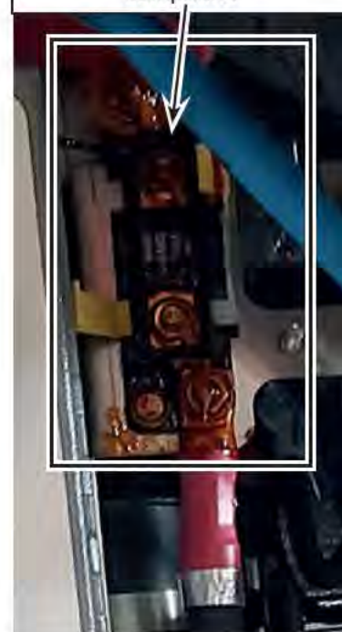
Figure 9 - Conform Application of N67314 NCP-2 Anticorrosive Compound
