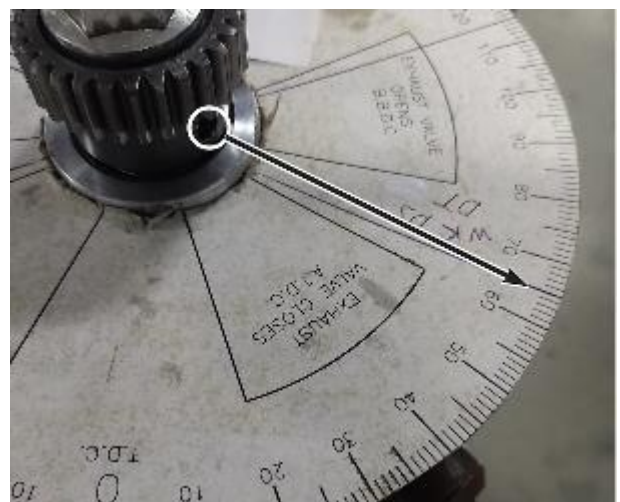
Figure 37 – Installing a Printed Paper Degree Wheel from the Internet
