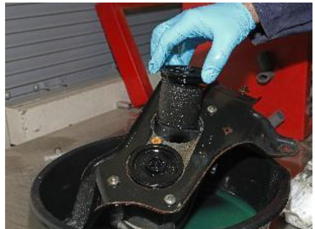
Figure 26 – Remove Old Filter Covers and Elements
