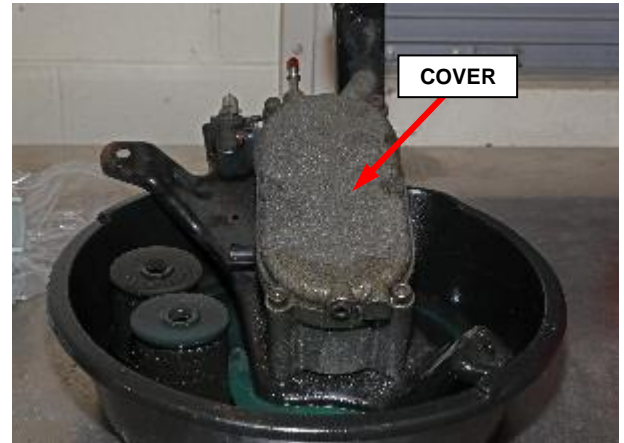
Figure 55 – Remove Fuel Filter/Water Separator Cover
