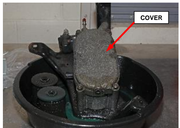
Figure 27 – Remove Fuel Filter/Water Separator Cover
