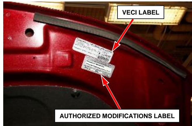
Figure 65 – Apply Authorized Modifications Label Near VECI Label (Specific Vehicle May Look Different)
