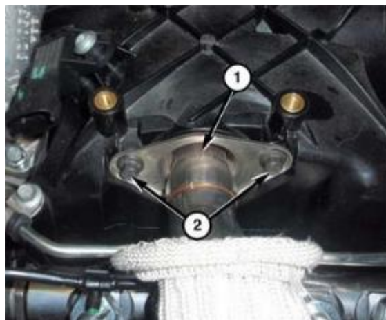
Figure 10 – Upper EGR Tube Bolts at Intake
