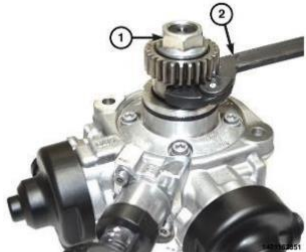
Figure 39 – HPFP Gear Removal
