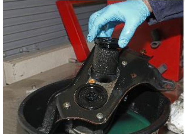
Figure 26 – Remove Old Filter Covers and Elements
