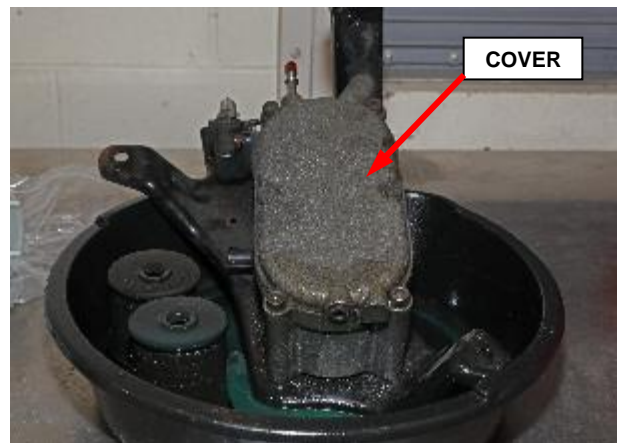
Figure 27 – Remove Fuel Filter/Water Separator Cover
