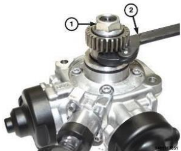
Figure 88 – Spanner Wrench and Drive Gear on the HPFP
