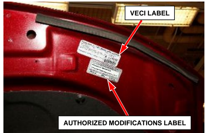
Figure 65 – Apply Authorized Modifications Label Near VECI Label (Specific Vehicle May Look Different)
