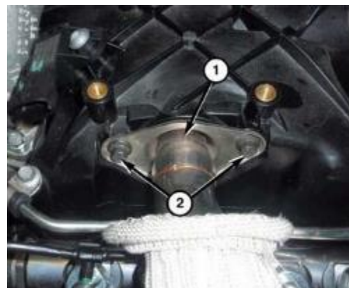
Figure 31 – Upper EGR Tube Bolts at Intake
