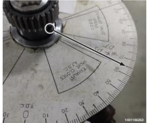
Figure 15 – Installing a Printed Paper Degree Wheel from the Internet
