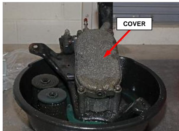
Figure 55 – Remove Fuel Filter/Water Separator Cover
