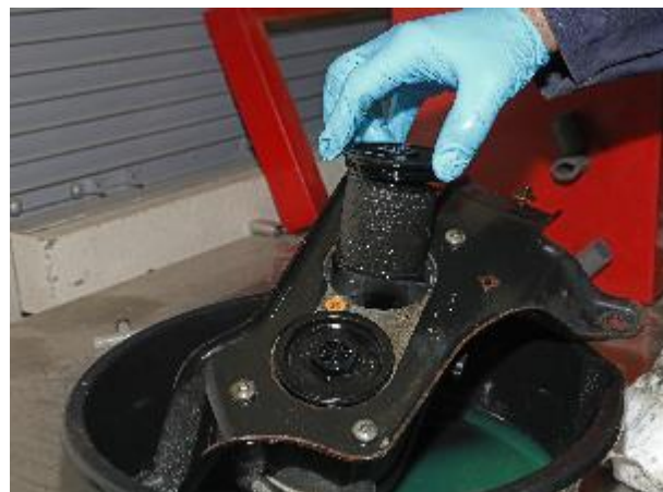
Figure 1 – Remove Old Filter Covers and Elements
