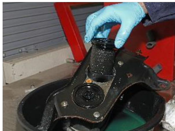
Figure 26 – Remove Old Filter Covers and Elements
