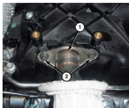
Figure 31 – Upper EGR Tube Bolts at Intake
