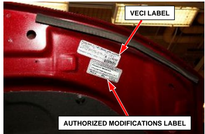
Figure 91 – Apply Authorized Modifications Label Near VECI Label (Specific Vehicle May Look Different)
