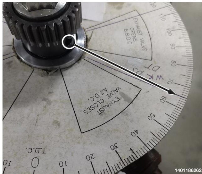
Figure 73 – – Installing a Printed Paper Degree Wheel from the Internet
