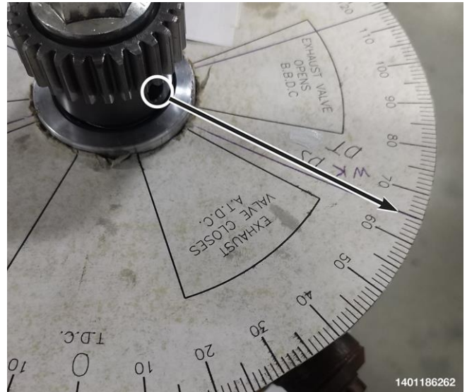
Figure 85 – – Installing a Printed Paper Degree Wheel from the Internet
