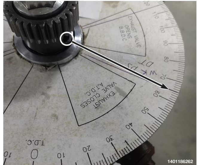
Figure 64 – Installing a Printed Paper Degree Wheel from the Internet
