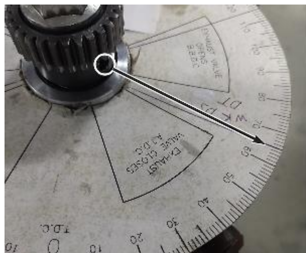
Figure 26 – Installing a Printed Paper Degree Wheel from the Internet
