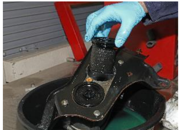
Figure 26 – Remove Old Filter Covers and Elements
