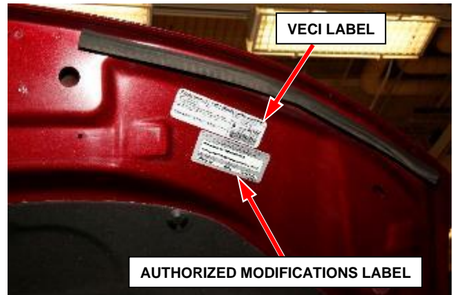
Figure 91 – Apply Authorized Modifications Label Near VECI Label (Specific Vehicle May Look Different)
