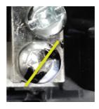
If the PoN connector <u>DOES MOVE</u>, the clamping screw in the PoN connector must be tightened.
