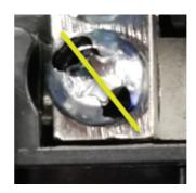
If the PoN connector <u>DOES MOVE</u>, the clamping screw in the PoN connector must be tightened.
