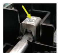
b. Tighten the clamping screw 1/4 turn at a time, <u>verifying for movement after each 1/4 turn</u>, until the connector does not move anymore. When the connector will not move anymore, apply a mark with the black permanent marker, between the connector and clamping screw. See Figure 10.
