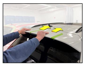
Starting from the middle to the outer edges, work your way along the spoiler pressing firmly to secure the spoiler once the spoiler is correctly positioned.
