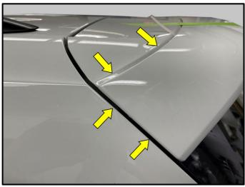
When installing the spoiler, ensure the gaps and body seam distances are even on both sides of the vehicle.
