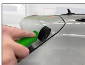
Using tool -T40400- (or equivalent) roll all of the exterior contact edges (double sided tape to body) with a force of 70-100N to fully seat the double sided tape.
