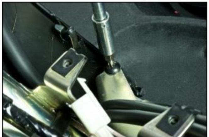
Remove the dashboard trim panel, unscrewing the 2 fastener screws.
