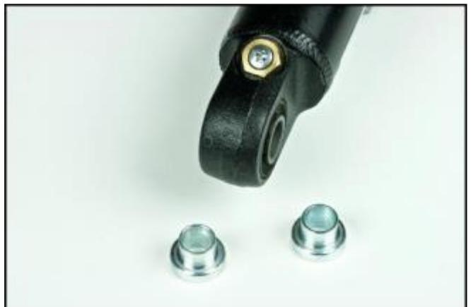
Remove the screw with the washer.
