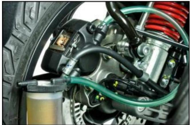
N.B: The photo illustrates the position of the steering where the reservoir of the front master cylinder offers the best filling conditions.
