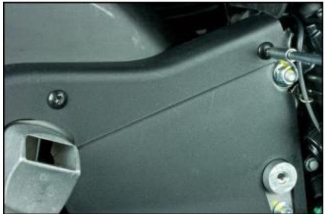
Remove the speed sensor, unscrewing the 2 fastener screws.
