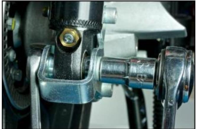
Remove the upper fastener bolt of the shock absorber.
