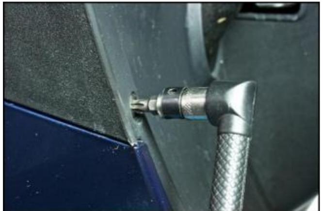
Remove the lower fastener screw of the right hand footboard.
