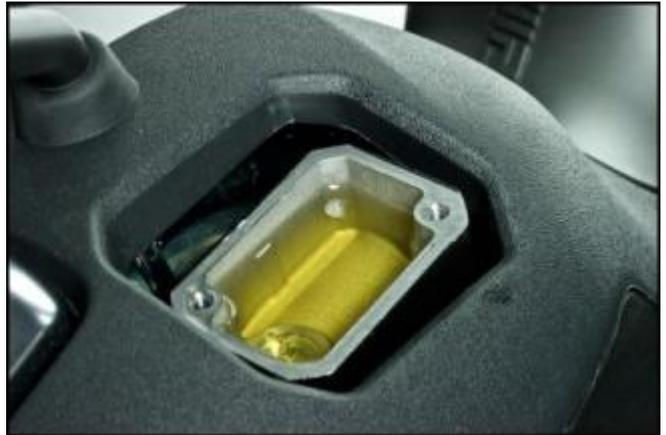
Continue filling the rear brake circuit until approximately 120 cc has been drained into the collector container.
