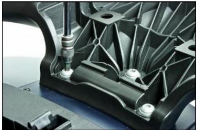
Remove the 2 screws fastening the rear cover.
