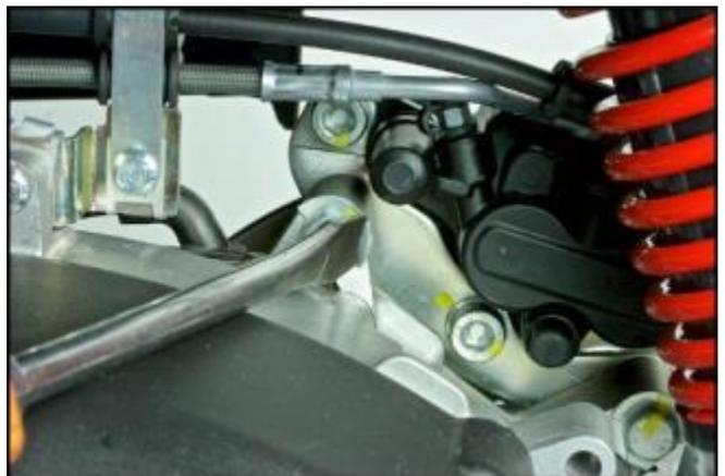
Remove the 2 fastener screws complete with anti-rotation devices.
