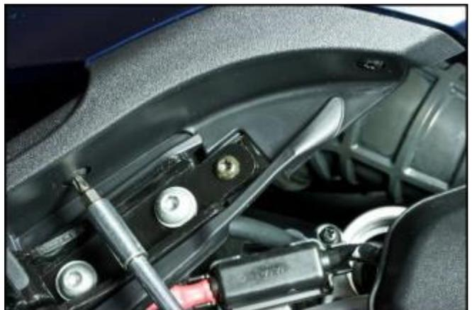
Remove the 2 screws fastening the centre cover, near the saddle.
