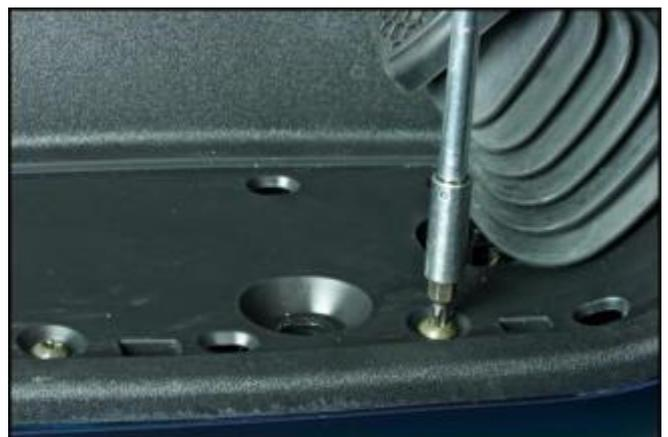
Lift up the gaiter and remove the upper part of the combined braking system pedal, unscrewing the 2 fastener screws.
