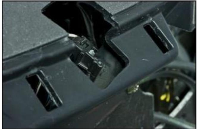
Remove the 2 rear fastener screws of the dashboard.
