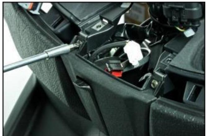
Remove the centre fastener screw of the cover panel.
