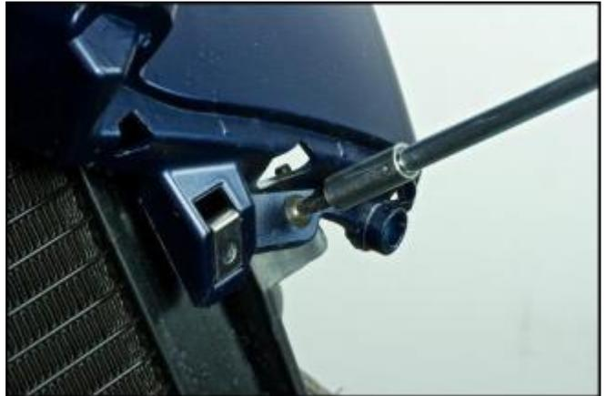
Remove the 2 upper fastener screws of the leg shield.
