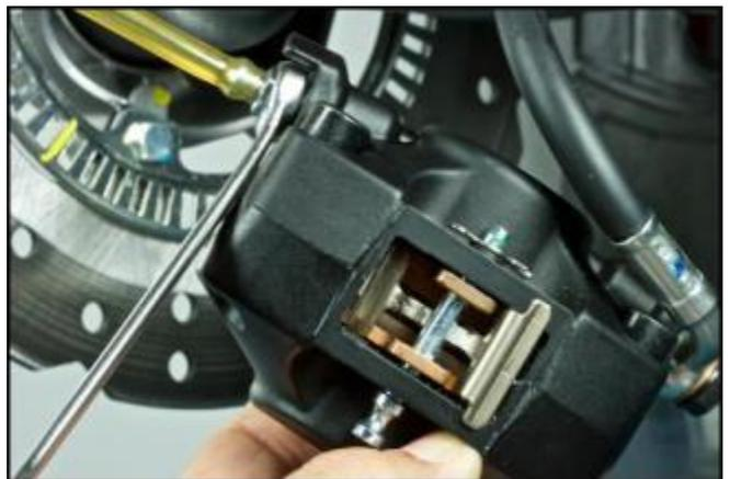
Refit the right hand calliper, tightening the 2 screws to a torque of 22 - 27 Nm.
