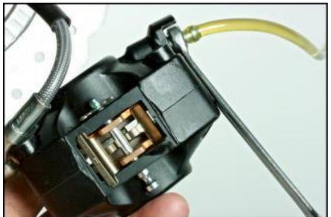
Refit the left hand calliper, tightening the 2 screws to a torque of 22 - 27 Nm.
