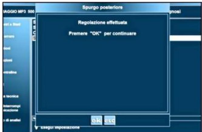
If the ABS modulator had had air inside, this would have been transferred into the lines between the ABS pump and the caliper.
