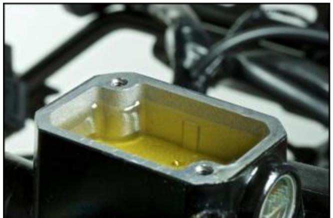
Close the lid of the reservoir, wiping off any spilt fluid.
