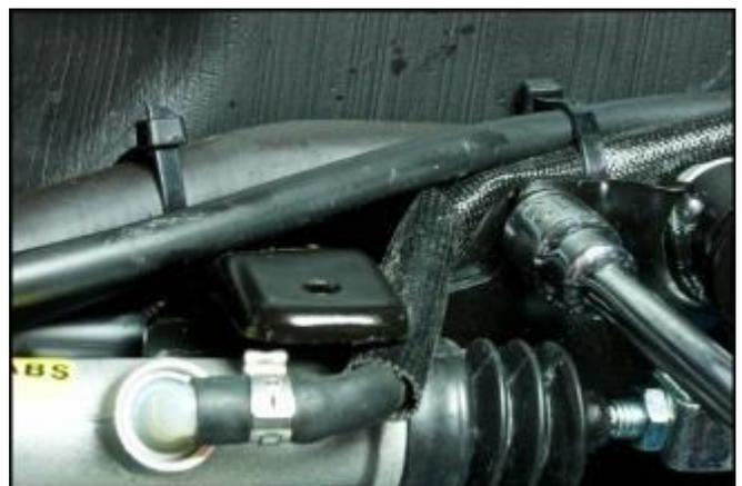
Remove the fastener screw of the combined braking system master cylinder reservoir and top up to the max. level.
