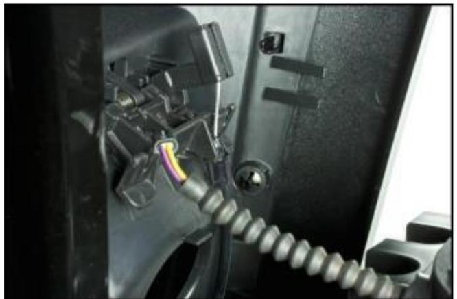
Remove the fastener plate of the right hand floor mat, unscrewing the 3 fastener screws.
