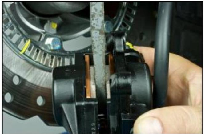
Hold the right hand calliper in a vertical position and pressurise the master cylinder.
