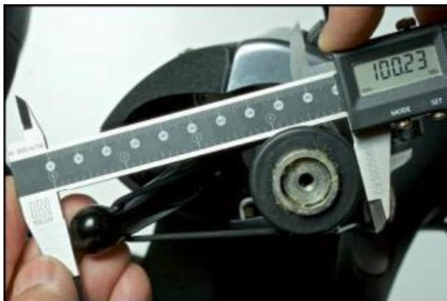
N.B: The measurement must be made with the vernier calliper perfectly aligned with the direction of movement of the lever.
