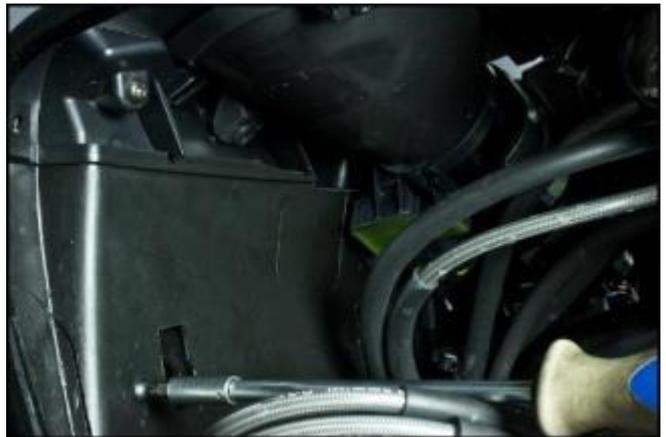
Remove the fastener screw of the expansion tank cap access cover.
