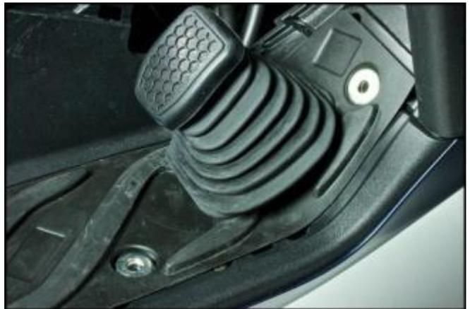
Remove the front fastener screw of the right hand footboard.
