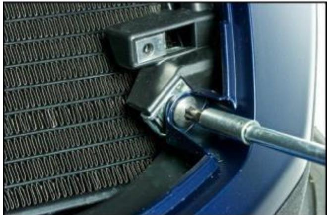
Remove the 2 upper screws fastening the bodywork mount.
