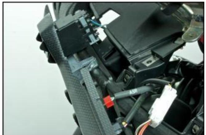
Remove the cover of the bag holder hook, unscrewing the 2 fastener screws.
