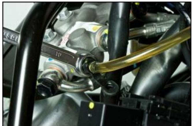
Refit the bracket of the combined braking system master cylinder, tightening the 3 screws to a torque of 20 Nm.
