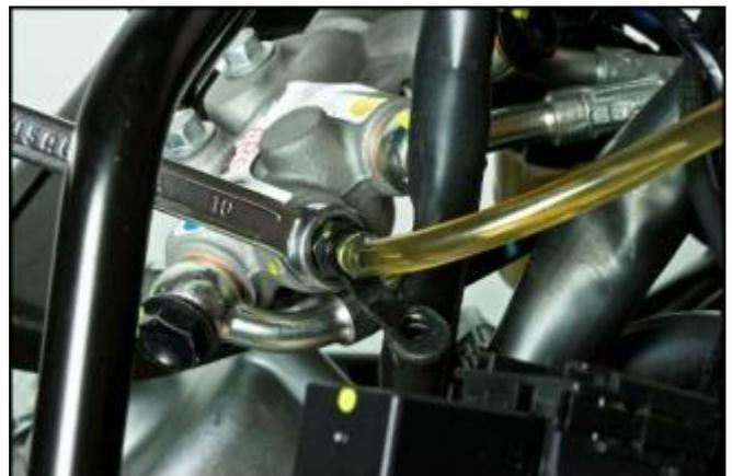
Once the pedal circuit has been bled completely, carry out the procedure to Replace all the brake fluid.
