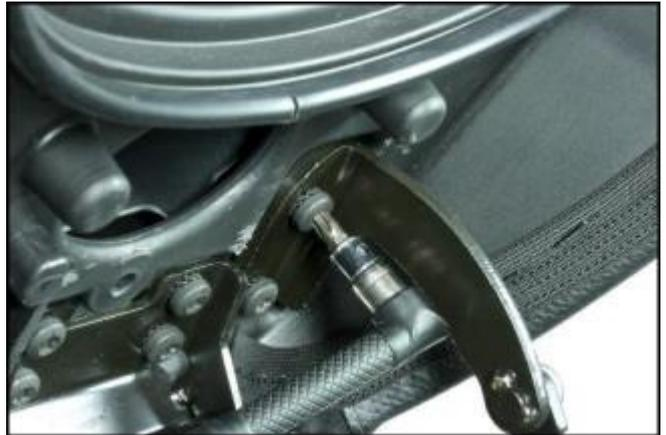
Remove the fastener screw and the cover of the internal saddle sensor.
