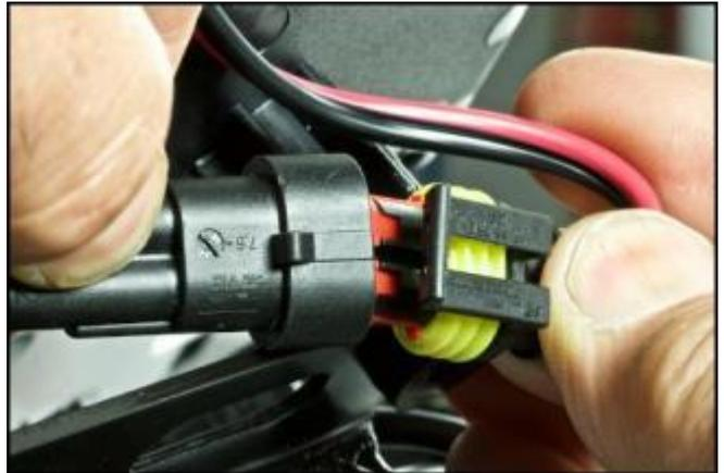
Release the lock tab and disconnect the flying lead connector of the dashboard connector.
