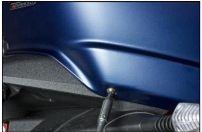
On both flanks, remove the 2 screws near the passenger footpegs.
