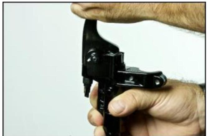
Refit the rear master cylinder onto the handlebar, making sure that the handlebar clamp U-bolt is fitted the right way around and that the clamp itself is adjusted correctly.
