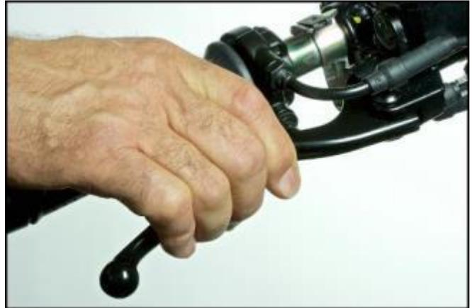
Pull the front brake lever and hold in position by fitting the O-ring, p/n 006731, onto the lever and handgrip as shown in the photo.
