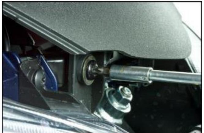
Remove the windscreen mount, removing the remaining 4 fastener screws with the relative shaped spacers.
