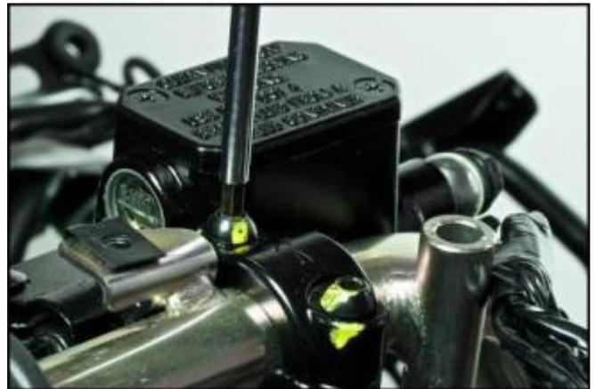
Hold the rear brake master cylinder in a vertical position. Pull the brake lever repeatedly while tilting the master cylinder slightly away from the vertical in all directions. Continue until there is the available travel of the lever reduces perceptibly.
