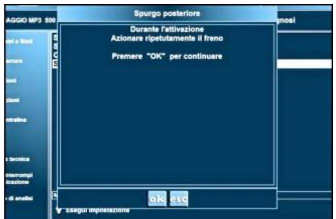
Command the activation of the valves of the rear channel.
