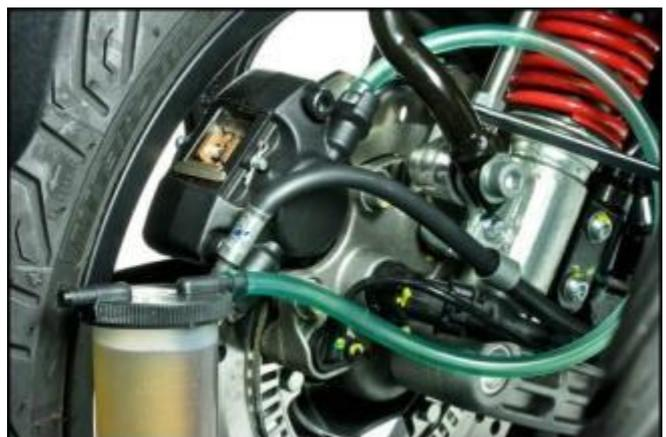
After bleeding the braking circuits and changing the brake fluid, reassemble the parts removed from the vehicle by following the steps for removal in reverse order.
