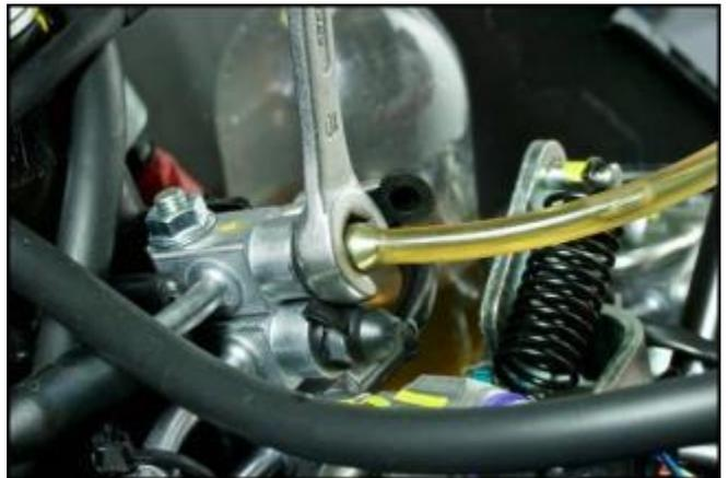
Top up the reservoir and bleed using the bottom nipple for the right hand circuit.
