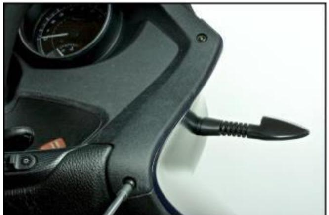
Remove the rear view mirrors, unscrewing and removing the fastener nuts with the relative washers.
