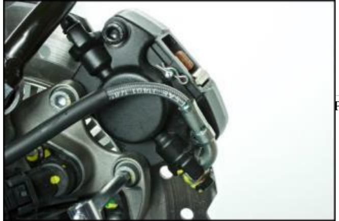
Remove the fastener screw of the right hand calliper pipe retainer clamp.
