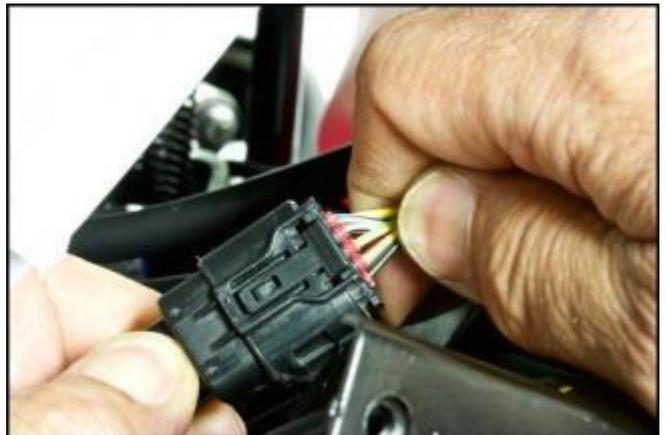
Release the lock tab and disconnect the dashboard connector.
