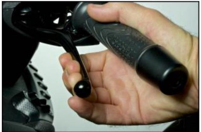
When the pressure of the electric pump prevails over the manual pump, maintain the pressure by reducing the stroke of the lever as necessary.
