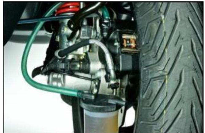
N.B: The photo illustrates the position of the steering where the reservoir of the front master cylinder offers the best filling conditions.
