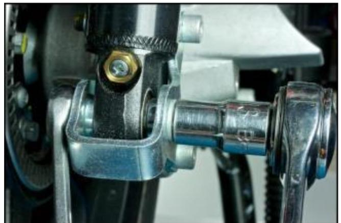
Remove the upper fastener bolt of the shock absorber.
