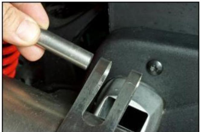
Remove the mounting screw of the silencer with the relative washers, and detach and remove the silencer from the exhaust pipe.
