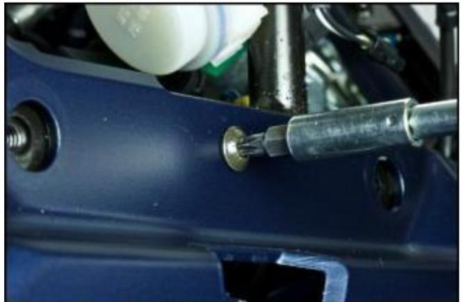
Remove the front leg shield, unscrewing the remaining 4 fastener screws.
