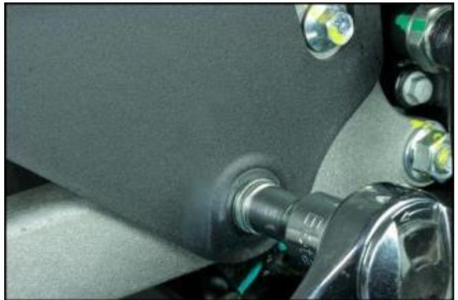
Remove the plastic guard panel, unscrewing the remaining 2 upper screws.
