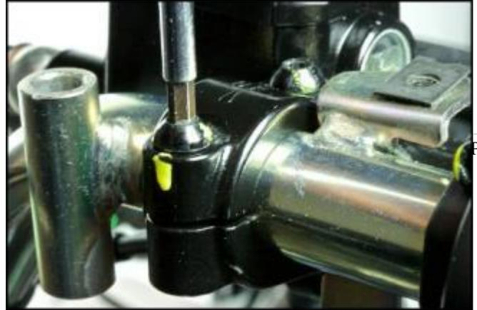
Manually check the effective travel of the front brake lever.
