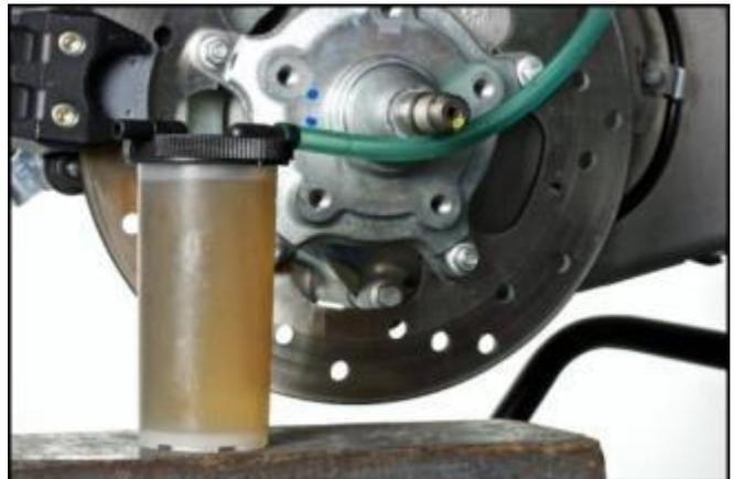
Fill the rear master cylinder reservoir to the max. level.
