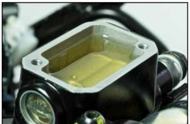
Fit the lid of the rear master cylinder reservoir, wiping off any spilt brake fluid.
