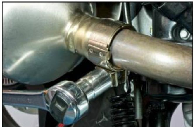
Loosen the check nut of the silencer fastener system.
