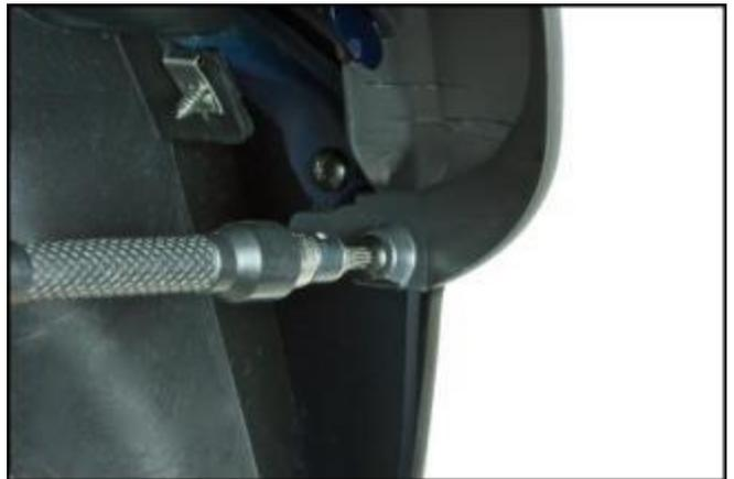
Remove the 2 fastener screws of the front cover, situated inside the wheel housings.
