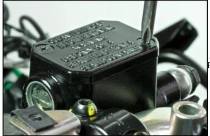
Disconnect the connectors of the brake switch. Remove the 2 screws and the handlebar clamp U-bolt.
