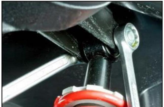
Remove the right hand shock absorber with the 4 spacers.
