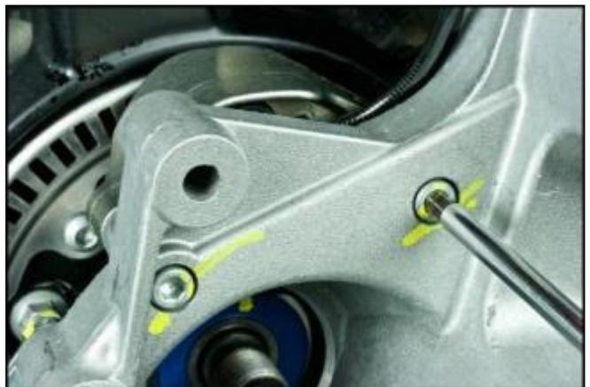
Remove the second fastener screw of the stand.
