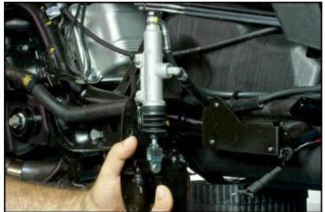
Connect the fluid collector container to the bleed nipple of the front brake servo pump and pump the pedal a few times while checking for air bubbles in the drained fluid.
