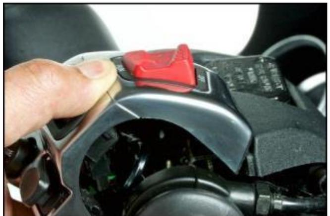
Remove the fastener screws of the handlebar cover, situated in the space under the handlebar switchgear sets
