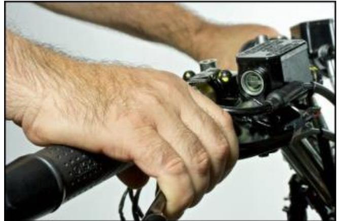
Press the combined braking system master cylinder pedal.
