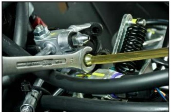
Remove the upper fasteners of both front callipers and restrain the callipers temporarily in a vertical position.
