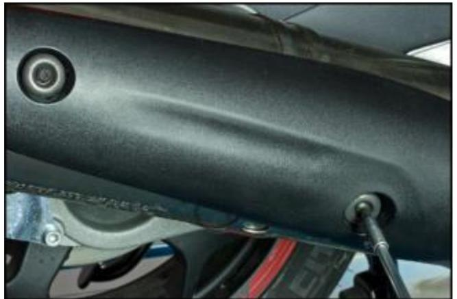
Loosen the screw of the metal clamp fastening the silencer to the exhaust pipe.
