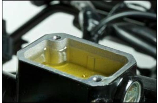
Continue filling the front brake circuit until approximately **120 cc** has been drained from the left front caliper into the collector container.
