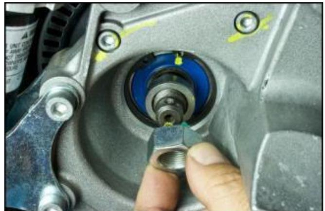
Pay attention to the correct positioning of the gasket and to the correct fastening of the slip joint clamp screw.
