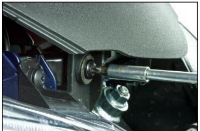
Remove the windscreen mount, removing the remaining 4 fastener screws with the relative shaped spacers.
