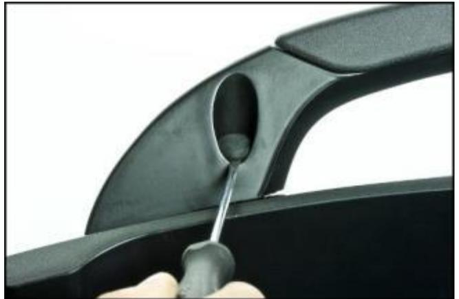
Remove the rear grab handle, undoing and removing the 5 screws with the relative washers.
