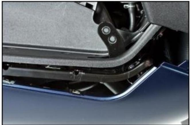
Check that the combined braking system pedal is against the retainer bracket of the brake light switch when the pedal itself in the rest position.
