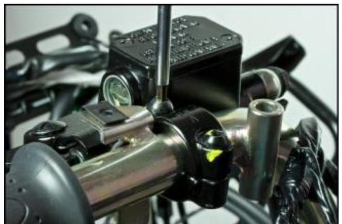
Manually check the effective travel of the rear brake lever.
