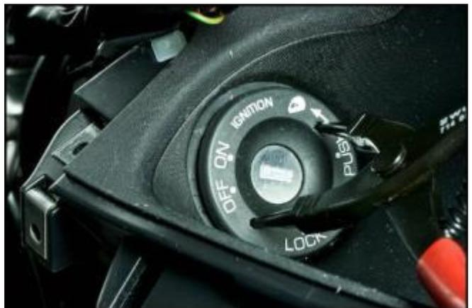
Remove the bezel of the ignition switch complete with metal ring.
