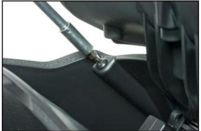
Remove the 2 front fastener screws of the windscreen mount complete with the relative washers.
