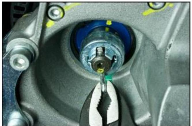
Engage the parking brake and remove the nut with the spacer.
