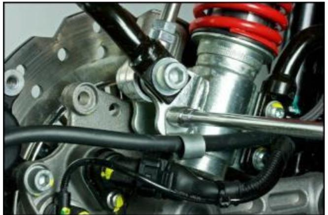
Remove the lower fastener screw of the right hand calliper and separate the pads, pushing the pistons to their respective end stops.
