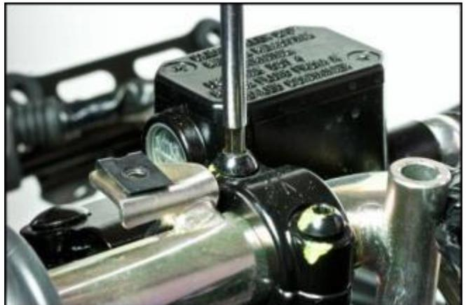
Remove the 2 screws and the lid of the reservoir complete with gasket.
