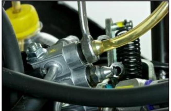
Repeat the step to check if the fluid drained from the upper bleed nipple of the right hand circuit contains air bubbles.
