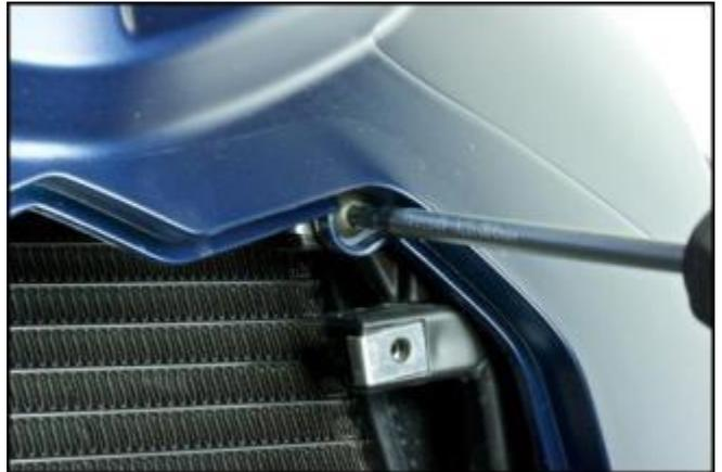
Remove the front cover, unscrewing the 2 Torx screws.
