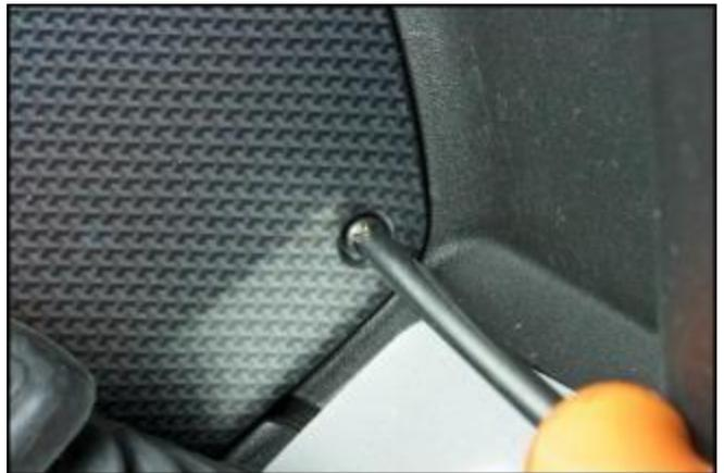
Remove the 2 fastener screws of the right hand centre cover.
