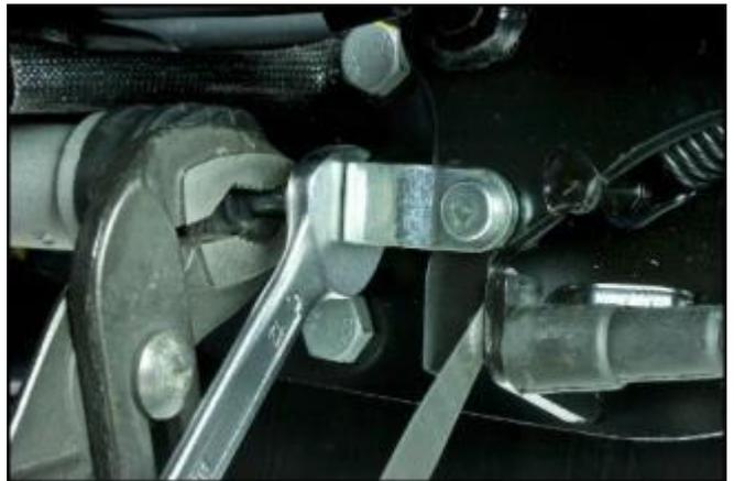
Remove the silencer guard, unscrewing and removing the 2 fastener screws with the relative metal flange rings.
