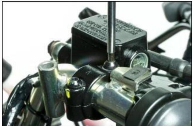
Rotate the right hand master cylinder into a vertical position.
