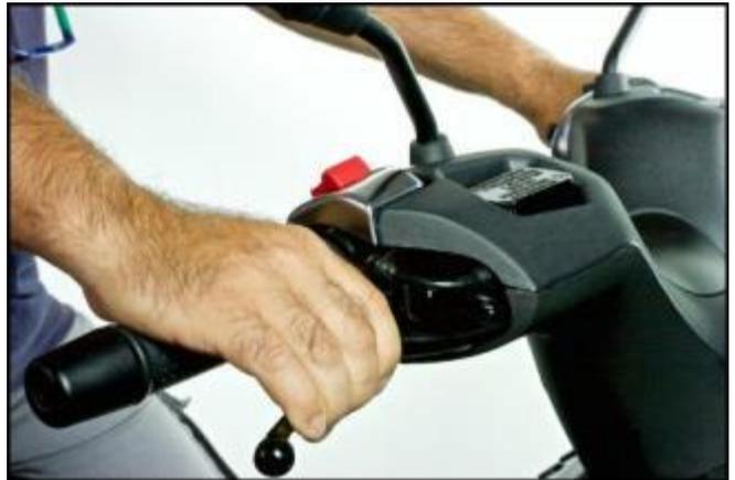
At the same time, press the combined braking system master cylinder pedal.
