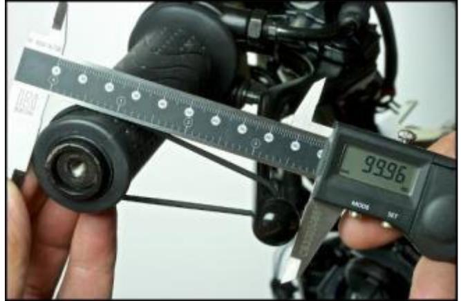
N.B: The measurement must be made with the vernier calliper perfectly aligned with the direction of movement of the lever.
