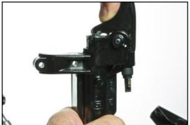
Refit the front master cylinder onto the handlebar, making sure that the handlebar clamp U-bolt is fitted the right way around and that the clamp itself is adjusted correctly.
