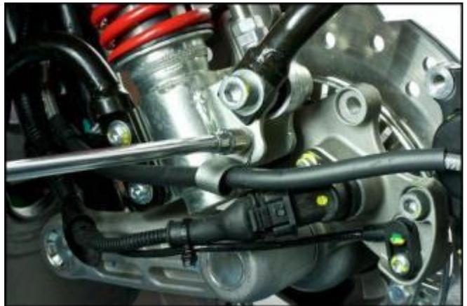
Remove the lower fastener screw of the left hand calliper and separate the pads, pushing the pistons to their respective end stops.
