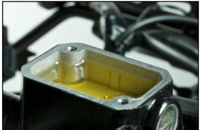
Continue filling the right front brake circuit until approximately **120 cc** has been drained from the right front caliper into the collector container.
