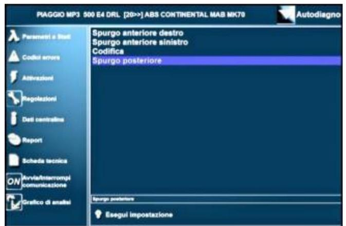
Before accessing the activation of the modulator, the message intended to prevent any unaware use of the modulator bleeding phase is displayed.
