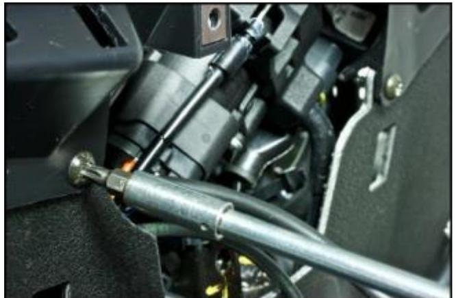
Using a pair of circlip pliers, turn the bezel of the ignition switch anticlockwise to align the word 'ON' with the key slot.
