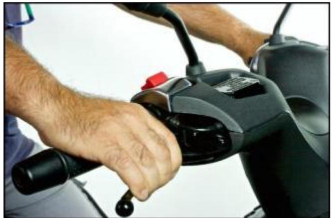
While holding the levers, check the travel of the combined braking system pedal.
