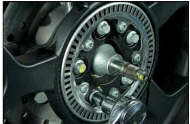
Continue with the reassembly of the carrier arm, paying attention to the correct application of all the tightening torques.
