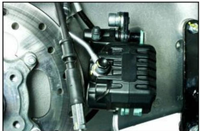
Pull the rear brake lever repeatedly to bring the brake pads into contact with each other.
