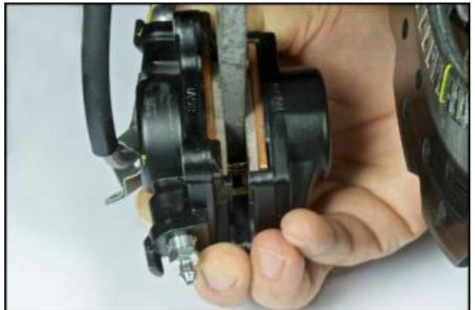
Hold the left hand calliper in a vertical position and pressurise the master cylinder.
