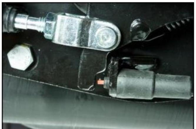
This is extremely dangerous as it may cause the rear brake circuit to remain under pressure even when the pedal is released
