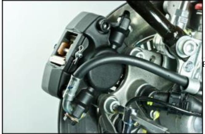
For greater safety, repeat the step to check if the fluid drained from the upper bleed nipple of the left hand circuit contains air bubbles.
