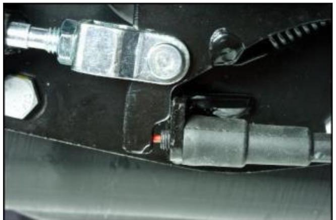
Press the pedal to release the brake light switch and reveal the clearance created between the **pedal arm** and the actuator pin of the brake light switch
