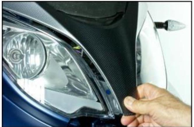
Remove the 2 fastener screws and the lower cover of the windscreen mount.
