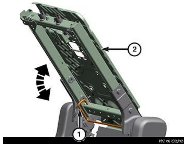
**Figure 62 – Seat Back Torsion Spring**
