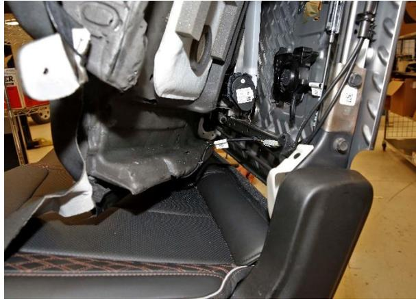
**Figure 74 – Electrical Connector**
