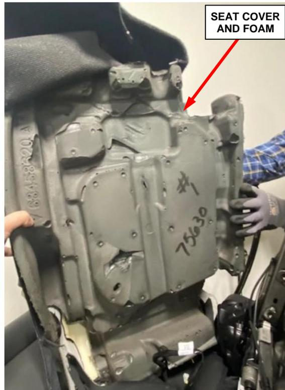
**Figure 31 – Seat Cover and Foam Assembly**
