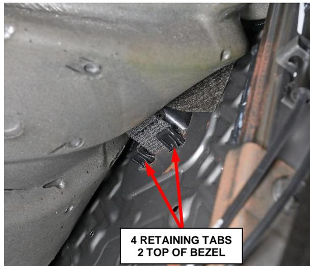
**Figure 6 – Bezel Retaining Tabs**
