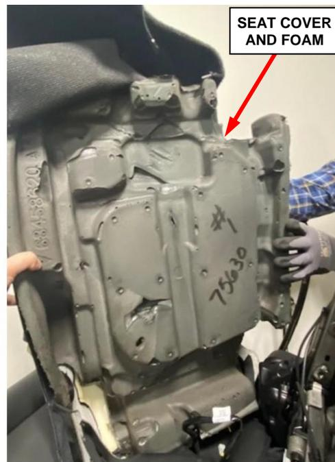
**Figure 58 – Seat Cover and Foam Assembly**
