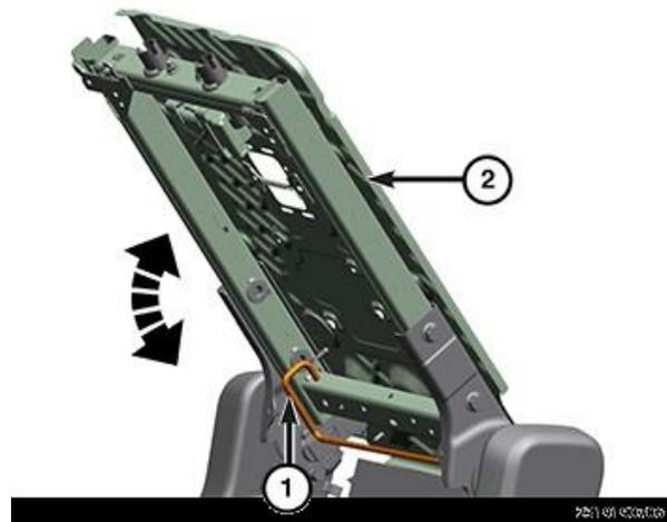
**Figure 85 – Seat Back Torsion Spring**
