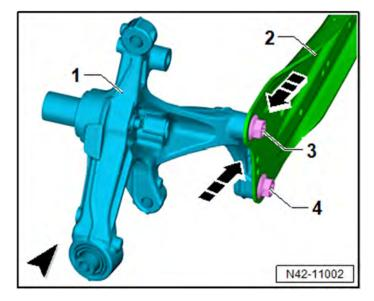
Torque trailing arm to wheel bearing housing bolts:
