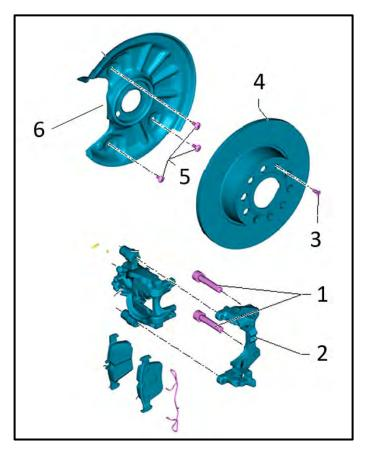
Reassemble brake components in the reverse order of removal:
