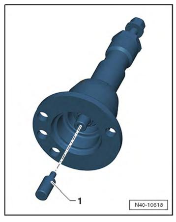
If the drive axle cannot be pulled out of the wheel bearing, then the drive axle can be pushed out of the wheel bearing using the Drive Shaft Remover -T10520A-.
