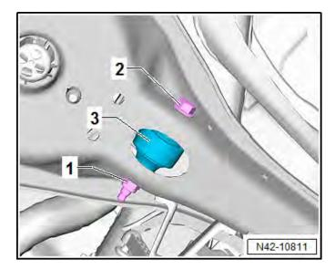
The upper spring support must be fully seated on the upper spring coil <arrow>.
