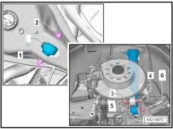
Counter-hold bolt <4> and torque nut <1> to 130 Nm + 180° in curb weight position.
