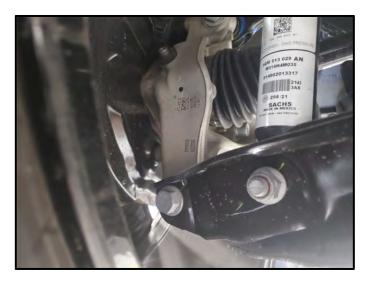
• Inspect rear wheel bearing housings and replace, if necessary.
