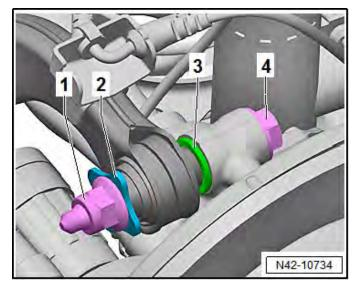
Disconnect wheel bearing housing and lower shock bolts from lower control arm and remove rear spring:
