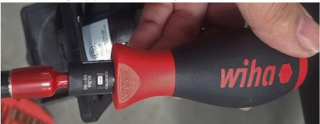
5. See photo below: There are 4 wire lugs on the inlet. You will need to verify the torque of these screws. They need to be tightened to 20 INCH LBS. If proper torque cannot be achieved due to the screw having the improper machining, the inlet must be replaced with a new one. If this is the case continue on to the next step.
