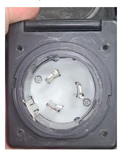
2. Remove the four #2 square head screws holding the inlet to the coach.
