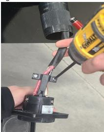
13. Verify the torque of the wire lugs @ 20 INCH LBS with torque screwdriver.
