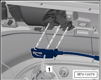
• Disconnect the cable <1> from the interior door mechanism.
