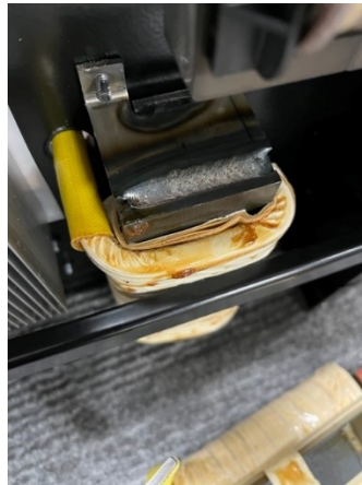
Incorrect Assembly (No Clearance)
